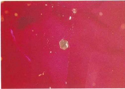
Fig. 3. Almost symmetrical, hexagonal metallic crystal with etched surface. Chatham ruby rough (189 ct). Transmitted and reflected light. 10x.
