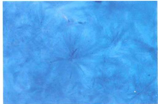
Fig. 2. Fibrous and radiating inclusions in blue devitrified glass imitating lapis lazuli.
