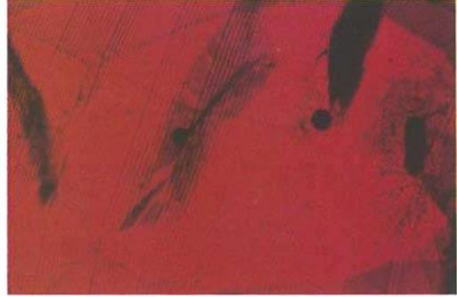
Fig. 16. Natural ruby from Thailand, intercalated lamellae of corundum in twin position on  $(10\bar{1}1)$ ; the lamellae showing interference striations. x pol., 30x.
