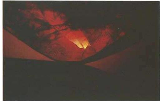
Fig. 41. Kashan synthetic ruby, one intercalated lamella of corundum in twin position on (1011) ends irregularly within the dominant crystal. x pol., 24x.
