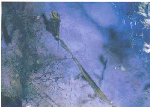
Fig. 7. Elongate, thin metallic blade (note 'feather' and white flux also). Chatham blue sapphire rough (45.8 ct). Transmitted and reflected light. 10x.
