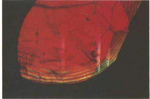
Fig. 38. Kashan synthetic ruby, intercalated lamellae of corundum in twin position on (1011). x pol., 40x.
