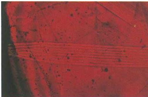
Fig. 13. Natural ruby from Sri Lanka, intercalated lamellae of corundum in twin position on  $(10\bar{1}1)$ ; the lamellae showing interference striations. x pol., 25x.
