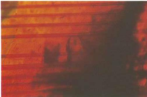
Fig. 19. Natural ruby from Sri Lanka, polysynthetic twinning on  $(10\bar{1}1)$ . Plane polarized light. 80x
