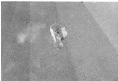
Fig. 3. Idiomorphic crystals of apatite with unidentified dark inclusions. 50x.
