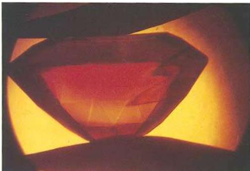
Fig. 5. Synthetic amethyst from new Japanese production; acute-angled twinned areas incorporated into the main crystal which is not twinned on the Brazil law. 16x.
