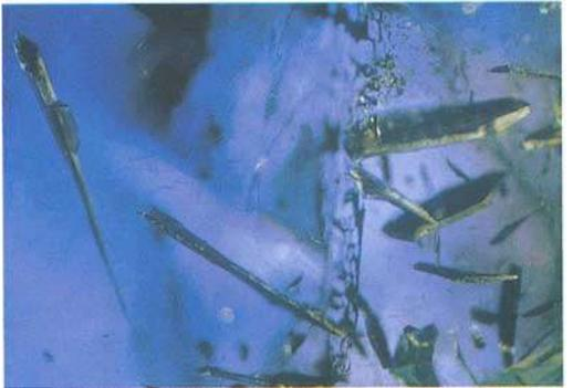
Fig. 6. Hexagonal plates, bars and dagger-like metallic inclusions. Chatham blue sapphire rough (45.8 ct). Transmitted and reflected light. 10x.
