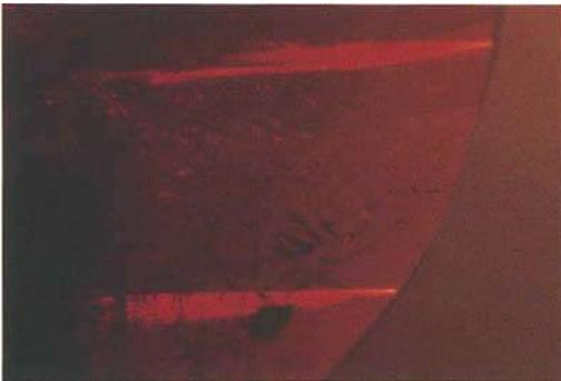
Fig. 35. Chatham synthetic ruby, intercalated lamellae of corundum in twin position on  $(10\bar{1}1)$ . x pol., 35x.
