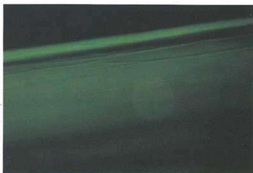
Fig. 16. The peaks and valleys of the 'mountain peak' feature seen in Figure 15 are revealed as long streaks passing along the length of the stone when viewed at right angles and through the girdle.
