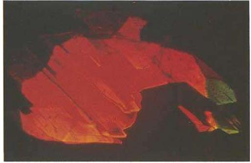
Fig. 25. Natural ruby from Thailand, intercalated lamellae of corundum in twin position on (1011) end irregularly within the dominant crystal. x pol., 35x.
