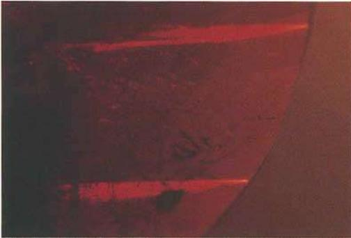
Fig. 35. Chatham synthetic ruby, intercalated lamellae of corundum in twin position on (1011). x pol., 35x.
