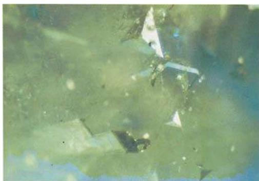
Fig. 11. Metallic pyramids, plates and irregular inclusions. Chatham blue sapphire crystal cluster (102 ct). Transmitted and reflected light. 16x.
