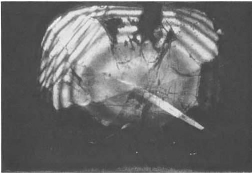
Fig. 36. Chatham synthetic ruby, intercalated lamellae of corundum in twin position on (1011) parallel to two rhombohedral faces. x pol., 20x.
