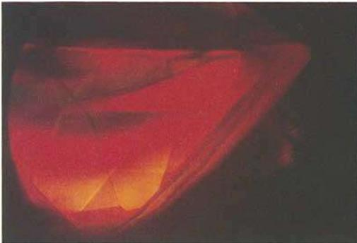
Fig. 3. Synthetic amethyst from new Japanese production; acute-angled twinned area incorporated into the main crystal which is not twinned on the Brazil law. Crossed polarizers. 24x.
