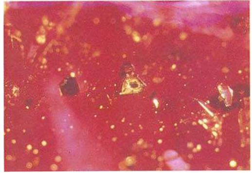
Fig. 2. Triangular inclusion (with attached white flux) pseudo-hexagonal and irregular metallic crystals. Chatham ruby crystal cluster (284 ct). Transmitted and reflected light. 16x.
