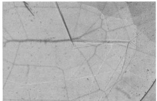
Fig. 42. Ramaura synthetic ruby, irregular structural surface. 30x.
