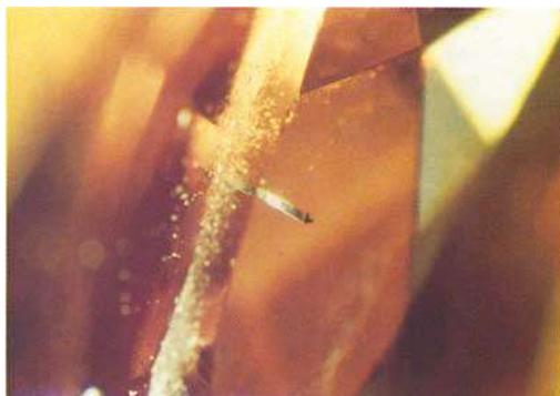
Fig. 10. Metallic bar with triangular cross-section immediately beneath girdle. Chatham orange-pink ('padparadscha' colour) faceted sapphire (0.89 ct). Transmitted and reflected light. 10x.
