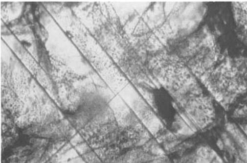
Fig. 40. Kashan synthetic ruby, intercalated lamellae of corundum in twin position on (1011) parallel to two rhombohedral faces. 50x.
