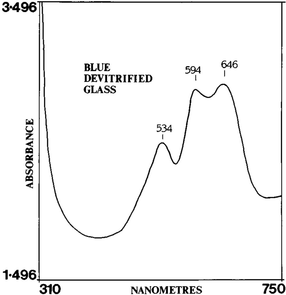
Fig. 3. The absorption curve of the blue devitrified glass in Figure 1. The curve was obtained using a Pye Unicam PU8800/03 UV/visible spectrophotometer (Basil Anderson model) with a speed of 1 nm/s and a bandwidth of 0.5 nm at room temperature. The path length was 0.5 mm.
