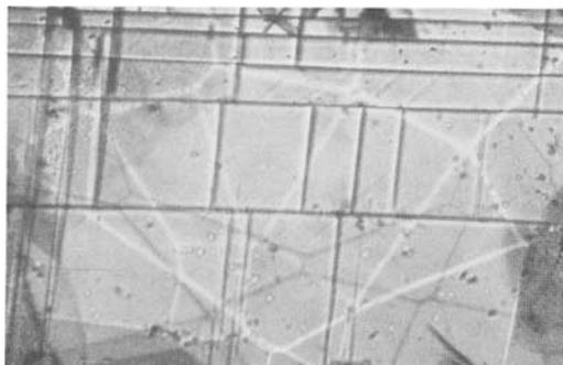
Fig. 22. Natural ruby from Thailand, intercalated lamellae of corundum in twin position on  $(10\bar{1}1)$  parallel to two rhombohedral faces; single lamellae end at other lamellae running through the crystal in nearly rectangular direction. 50x.
