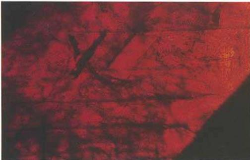
Fig. 39. Kashan synthetic ruby, intercalated lamellae of corundum in twin position on (1011). x pol., 45x.
