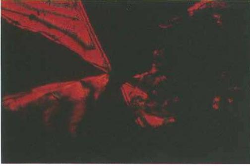
Fig. 3. Natural ruby from Sri Lanka, contact twin on  $(10\bar{1}1)$  with three crystals in twin position around a central crystal. x pol., 40x.
