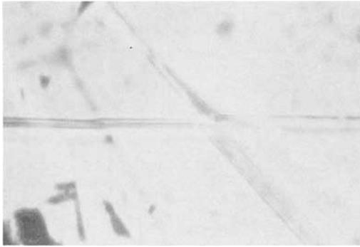
Fig. 33. Chatham synthetic ruby, intersecting structural planes (twin boundaries?). 95x.
