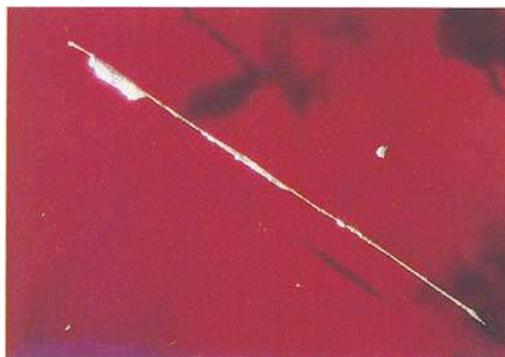
Fig. 9. Needle-like metallic inclusion coated with strongly reflecting white flux. Chatham ruby rough (189 ct). Transmitted and reflected light. 10x.
