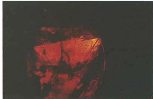
Fig. 23. Natural ruby from Burma, one intercalated lamella of corundum in twin position on  $(10\bar{1}1)$  ends irregularly within the dominant crystal. x pol., 32x.
