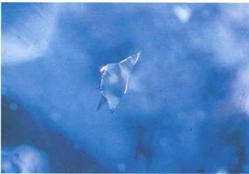
Fig. 12. Irregular silvery, metallic inclusion. Chatham blue sapphire rough (45.8 ct). Transmitted and reflected light. 10x.
