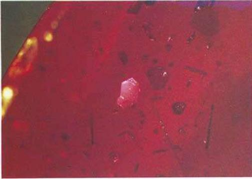
Fig. 1. Hexagonal plates (one strongly reflecting), triangles with truncated corners, bar and needle-like metallic inclusions. Chatham ruby cabochon (1.8 ct). Reflected light. 16x.
