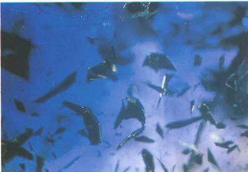
Fig. 5. Dense concentration of metallic blades, spicules, plates and irregular forms. Chatham blue sapphire rough (45.8 ct). Transmitted and reflected light. 10x.
