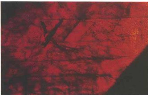
Fig. 39. Kashan synthetic ruby, intercalated lamellae of corundum in twin position on  $(10\bar{1}1)$ . x pol., 45x.
