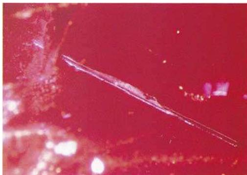
Fig. 8. Elongate metallic blade, partially coated with white flux. Chatham ruby rough (189 ct). Transmitted and reflected light. 10x.
