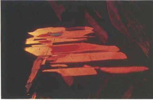
Fig. 24. Natural ruby from Thailand, intercalated lamellae of corundum in twin position on  $(10\bar{1}1)$  parallel to three rhombohedral faces end irregularly within the dominant crystal. x pol., 35x.
