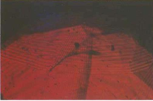
Fig. 15. Natural ruby from Burma, intercalated lamellae of corundum in twin position on  $(10\bar{1}1)$  parallel to two rhombohedral faces; the lamellae showing interference striations. x pol., 35x.
