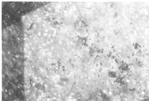
Fig. 1. The most common inclusions in corundum from Umba Valley are zircons. 25x.
