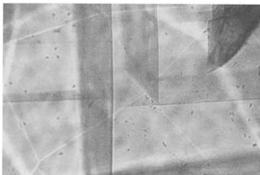
Fig. 20. Natural ruby from Thailand, intercalated lamellae of corundum in twin position on  $(10\bar{1}1)$  parallel to two rhombohedral faces; one lamella ends at another lamella running through the crystal in nearly rectangular direction. 50x.
