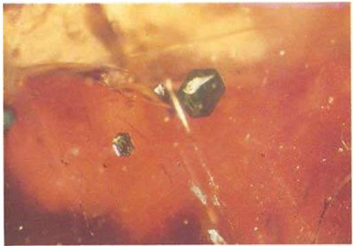
Fig. 4. Etched hexagonal metallic inclusions with some attached white flux. Chatham orange-pink ('padparadscha' colour) sapphire rough (425 ct). Reflected light. 10x.
