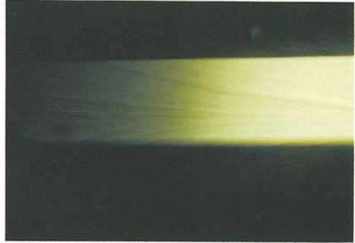
Fig. 15. A 'mountain peak' feature seen when looking down the optic axis of a 1.81 ct synthetic emerald.
