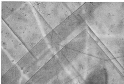
Fig. 21. Natural ruby from Thailand, intercalated lamellae of corundum in twin position on  $(10\bar{1}1)$  parallel to two rhombohedral faces; single lamellae end at other lamellae running through the crystal in nearly rectangular direction. 100x.
