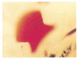
Fig. 3. Anhedral fragment of hematite in Eonyang amethyst from Korea. Growth planes intersecting at 120° are seen. Transmitted light. 200X.
