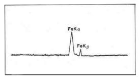
Fig. 5. Energy-dispersive spectrum of hematite inclusion in Eonyang amethyst from Korea.
