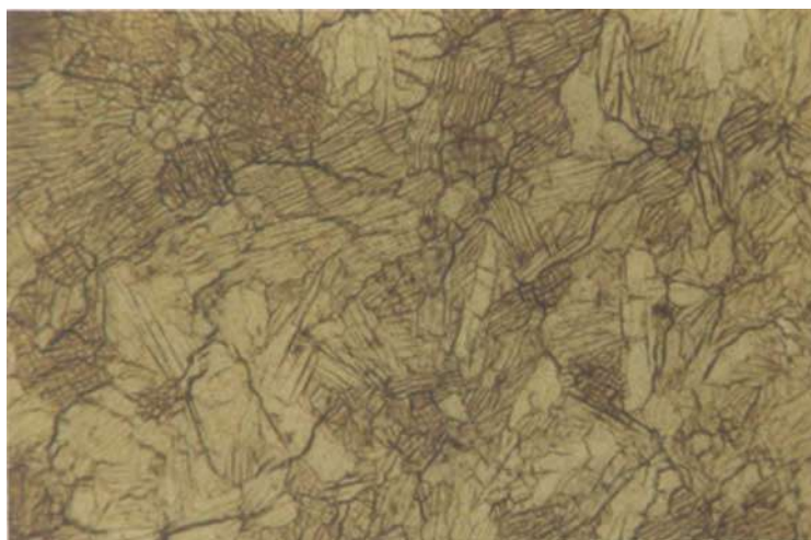
Fig. 2. Pure jadeite jade. Plane polarized light. x30.
