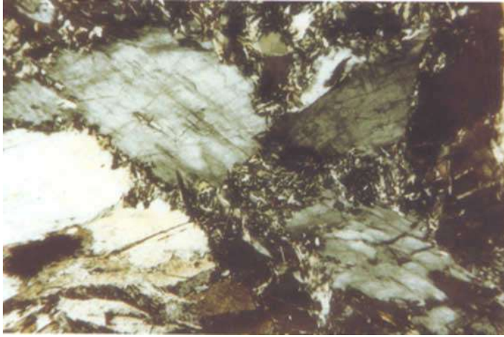
Fig. 5. Replacement of jadeite by actinolite along cleavage planes and boundaries. Crossed polars. x35.
