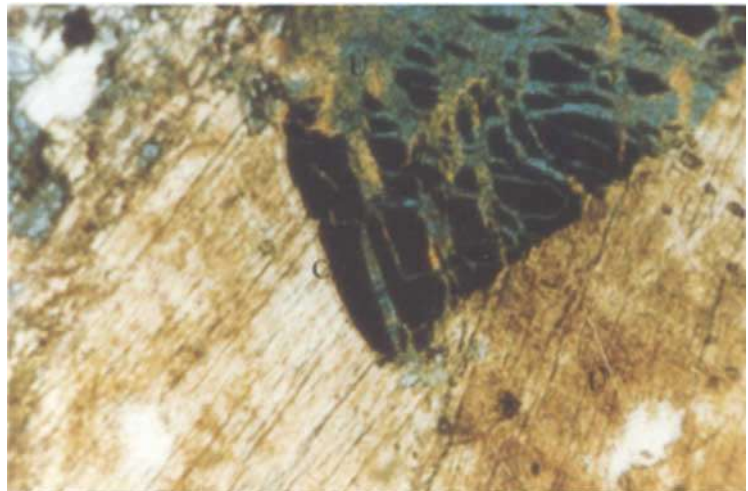
Fig. 10. Chromite and ureyite. Plane polarized light. \times 70 . Chromite (black), ureyite (green).
