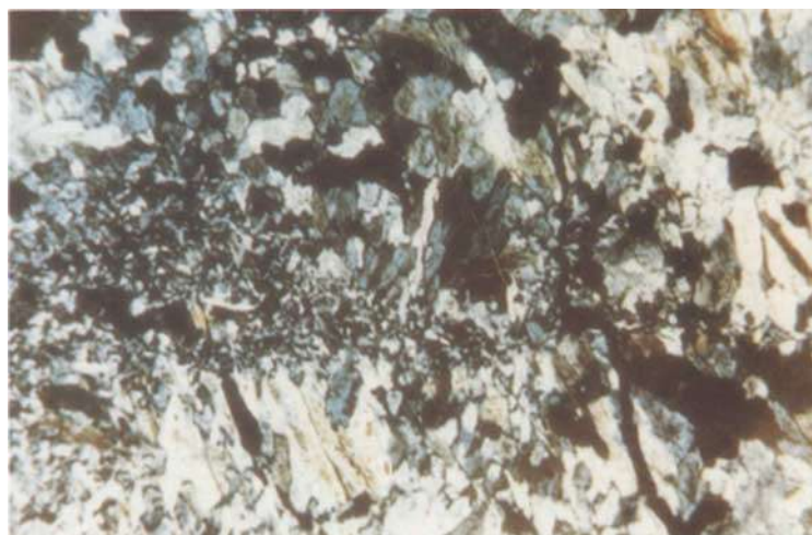
Fig. 3. Crushed jadeite jade. Crossed polars. x35.
