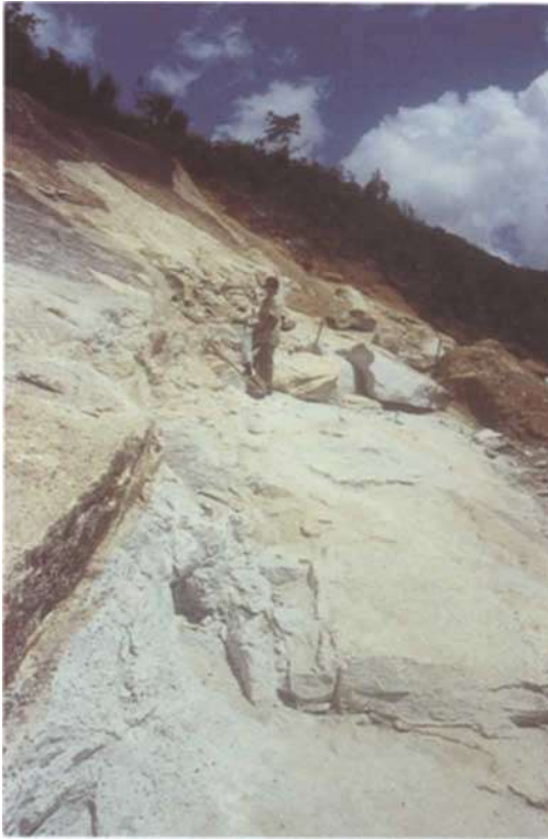
Fig. 17. Working a chrysoberyl-bearing pegmatite, during 1990, near Barro Preto (Minas Gerais State). The pegmatite may be seen along the small brown step in the foreground.
