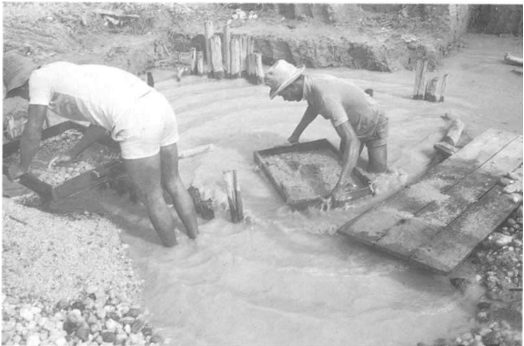
Fig. 12. Washing and sorting the chrysoberyl-bearing gravel. Rosalino prospect in the Córrego do Fogo alluvial deposit (Minas Gerais State).
