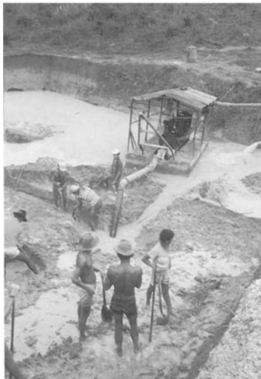
Fig. 13. Working an alluvial deposit by means of a small dredge, near Teófilo Otoni town (Minas Gerais State).
