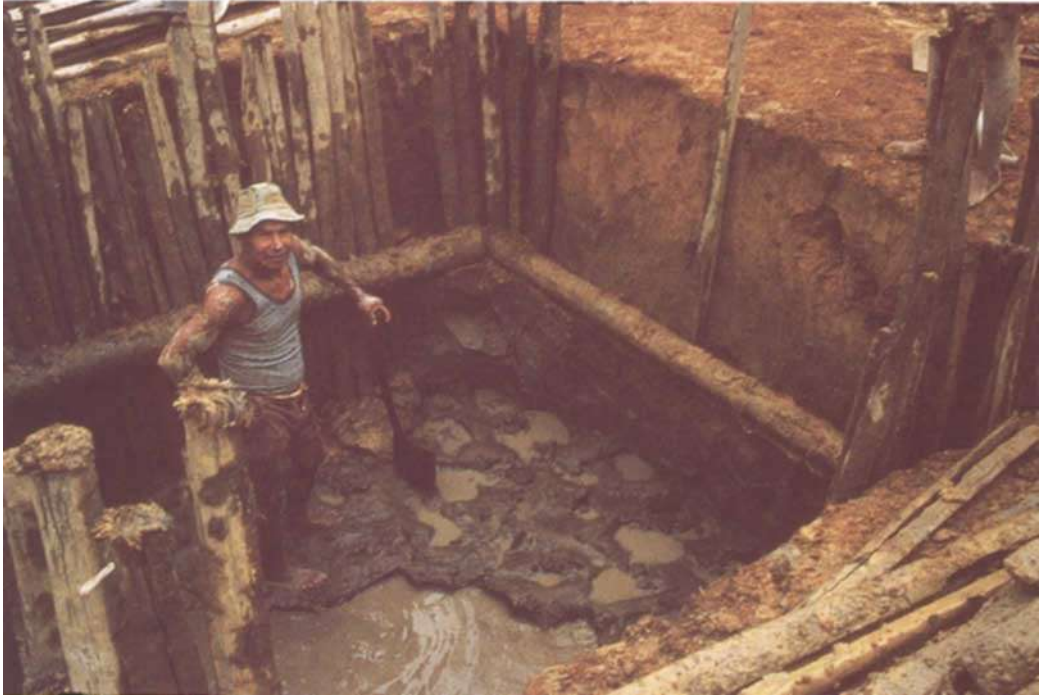
Fig. 11. Removing a pear horizon in the overburden. Córrego do Fogo alluvial deposit (Minas Gerais State).
