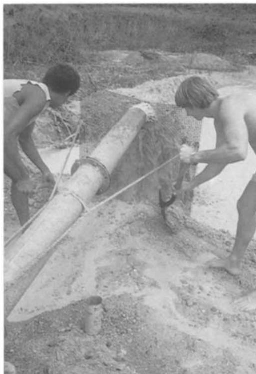
Fig. 14. Discharging the pumped chrysoberyl-bearing gravel. Gravel and pebbles are retained by the sieve before hand sorting. Medina alluvial deposit (Minas Gerais State).
