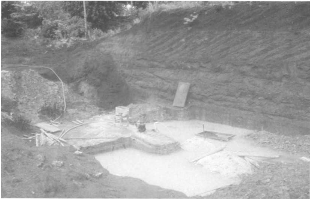
Fig. 15. After removing the thick reddish barren colluvium caused by sliding, workers found large V-twinned chrysoberyl crystals in the alluvial gravel of this flat in the Córrego Alegre (Dimão prospect – Espírito Santo State). See the 3 crystals in Figure 6.
