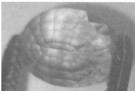
Fig. 1. Diffusion-treated Sri Lankan sapphire showing the spider-web effect produced by the concentration of colour at the facet edges
