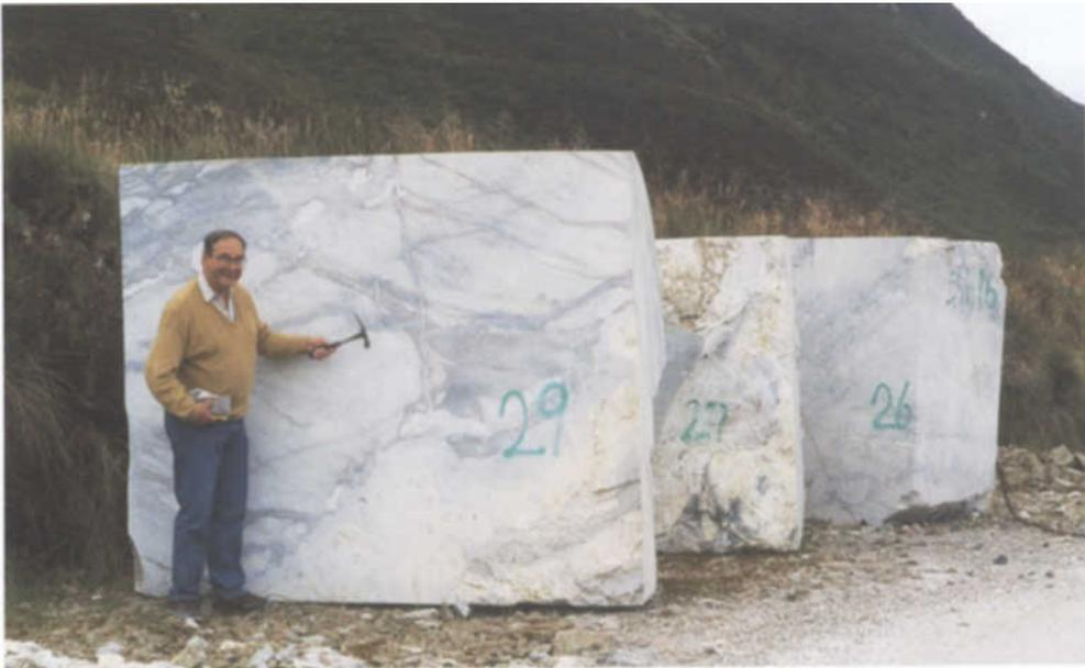
*Figure 5: Ledmore marble quarry. Slabs of grey architectural marble showing typical deformation textures. Photo by Douglas Nichol.*
