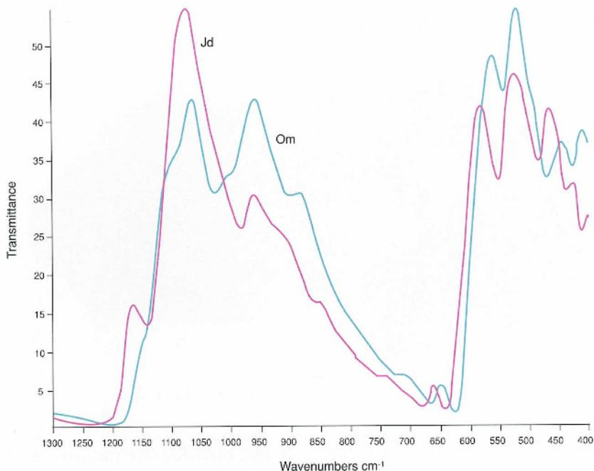
**Figure 5:** Infrared spectra of omphacite jade (Om) and jadeite jade (Jd).
