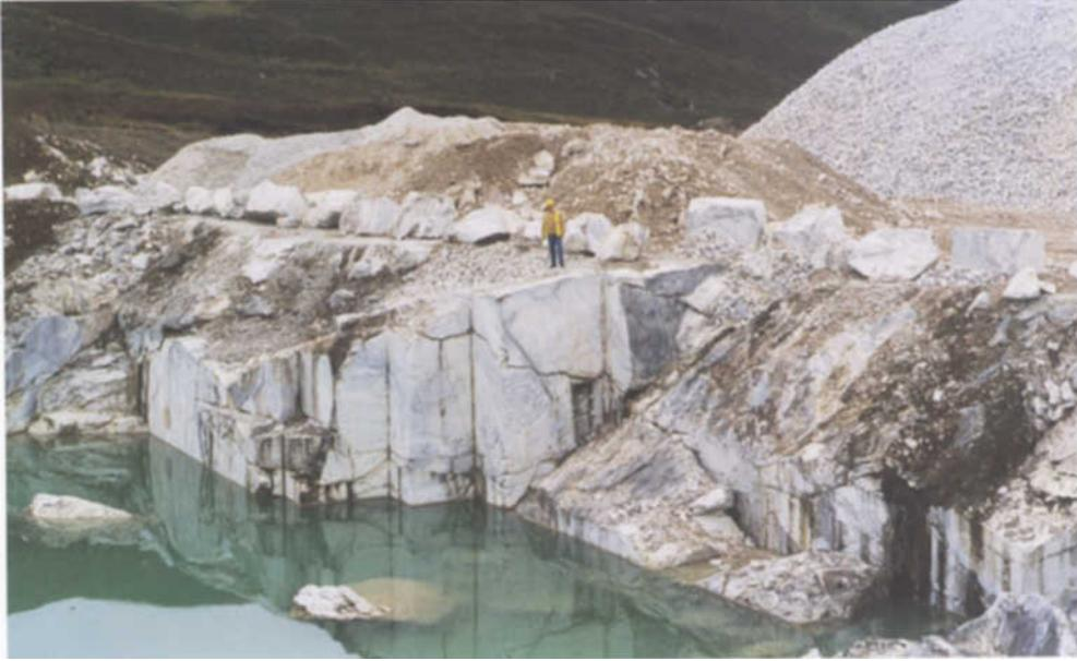
*Figure 4: Ledmore marble quarry. View looking westwards at wire-saw cut faces. Hills in the background consist of Cnoc na Sròine syenite. Photo by Douglas Nichol.*
