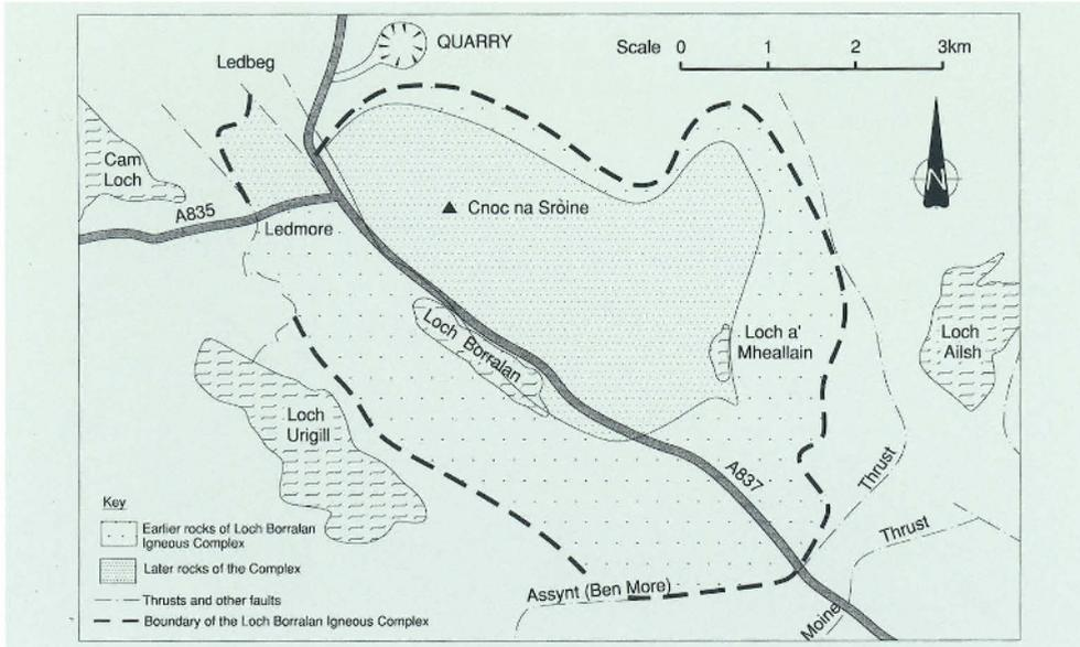
**Figure 2:** General Geology of the Ledmore area and the Loch Borrallan Igneous Complex. The country rock (unshaded) consists predominantly of Cambrian limestone and dolomite strata of the Durness Limestone Group.
