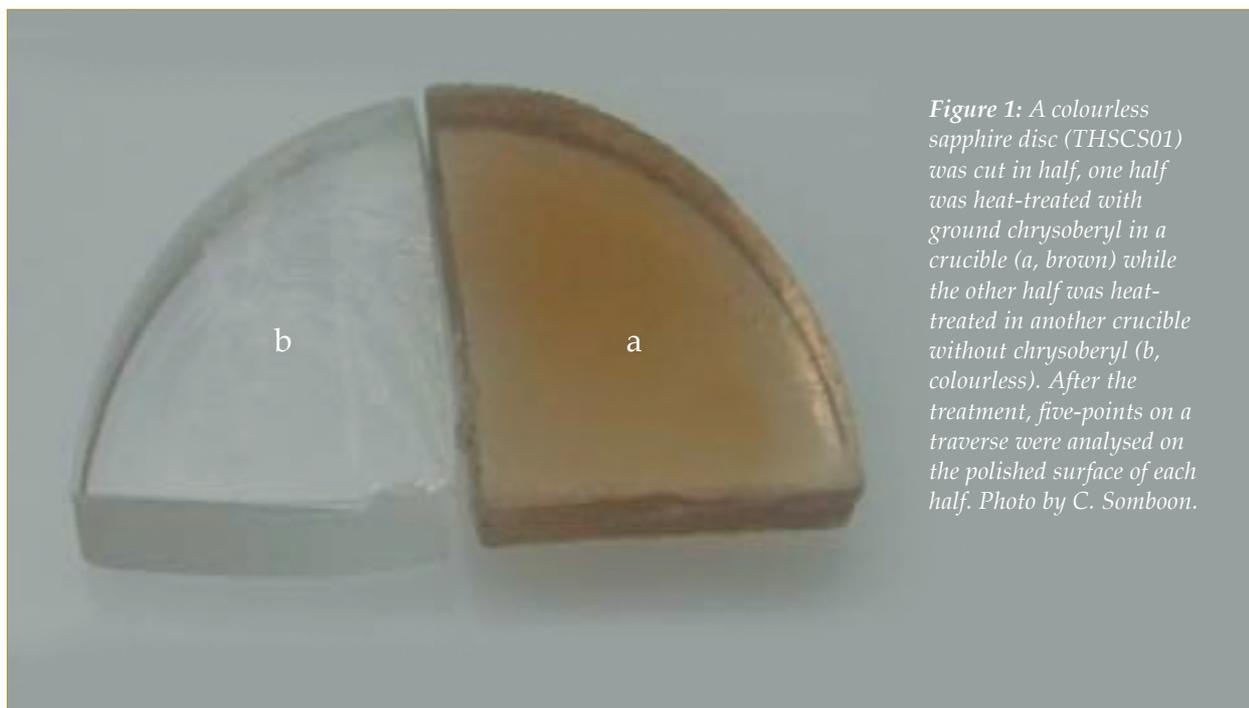
*Figure 1: A colourless sapphire disc (THSCS01) was cut in half, one half was heat-treated with ground chrysoberyl in a crucible (a, brown) while the other half was heat-treated in another crucible without chrysoberyl (b, colourless). After the treatment, five-points on a traverse were analysed on the polished surface of each half. Photo by C. Somboon.*
