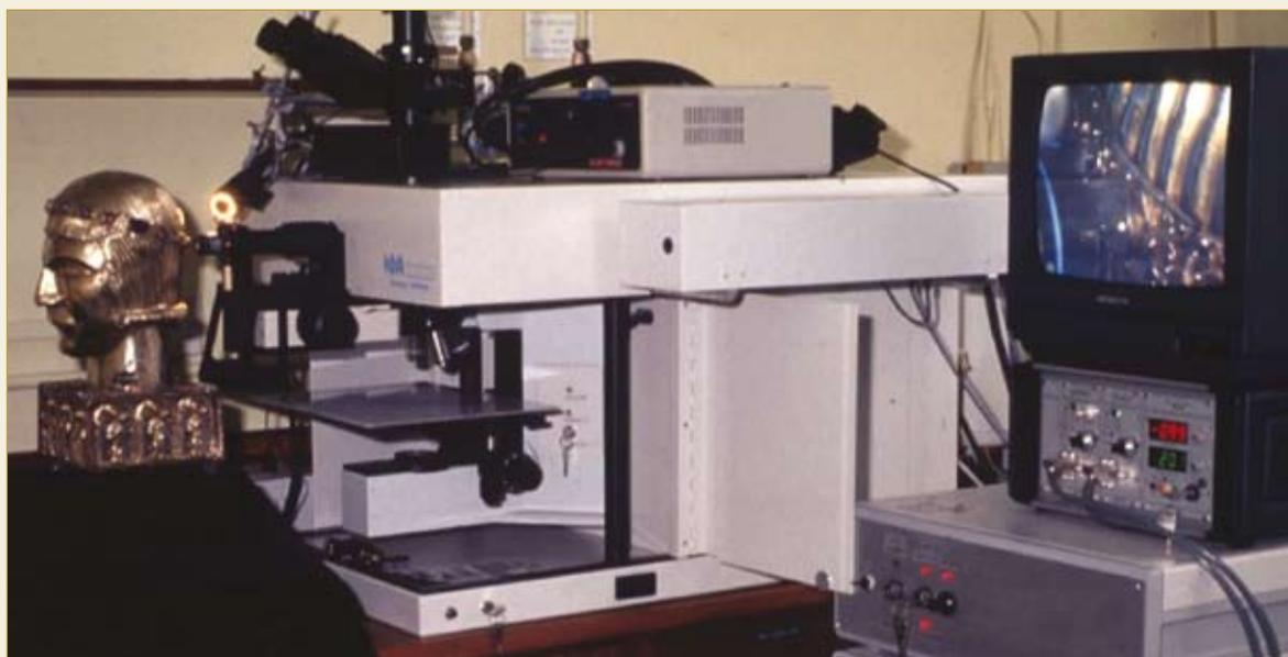
*Figure 3: The British Museum Raman microspectroscope with an open-beam horizontal microscope attachment showing how spectra were obtained from the gems on the head reliquary of St Eustace. A close-up image of part of the diadem is visible in the screen on the right.*
