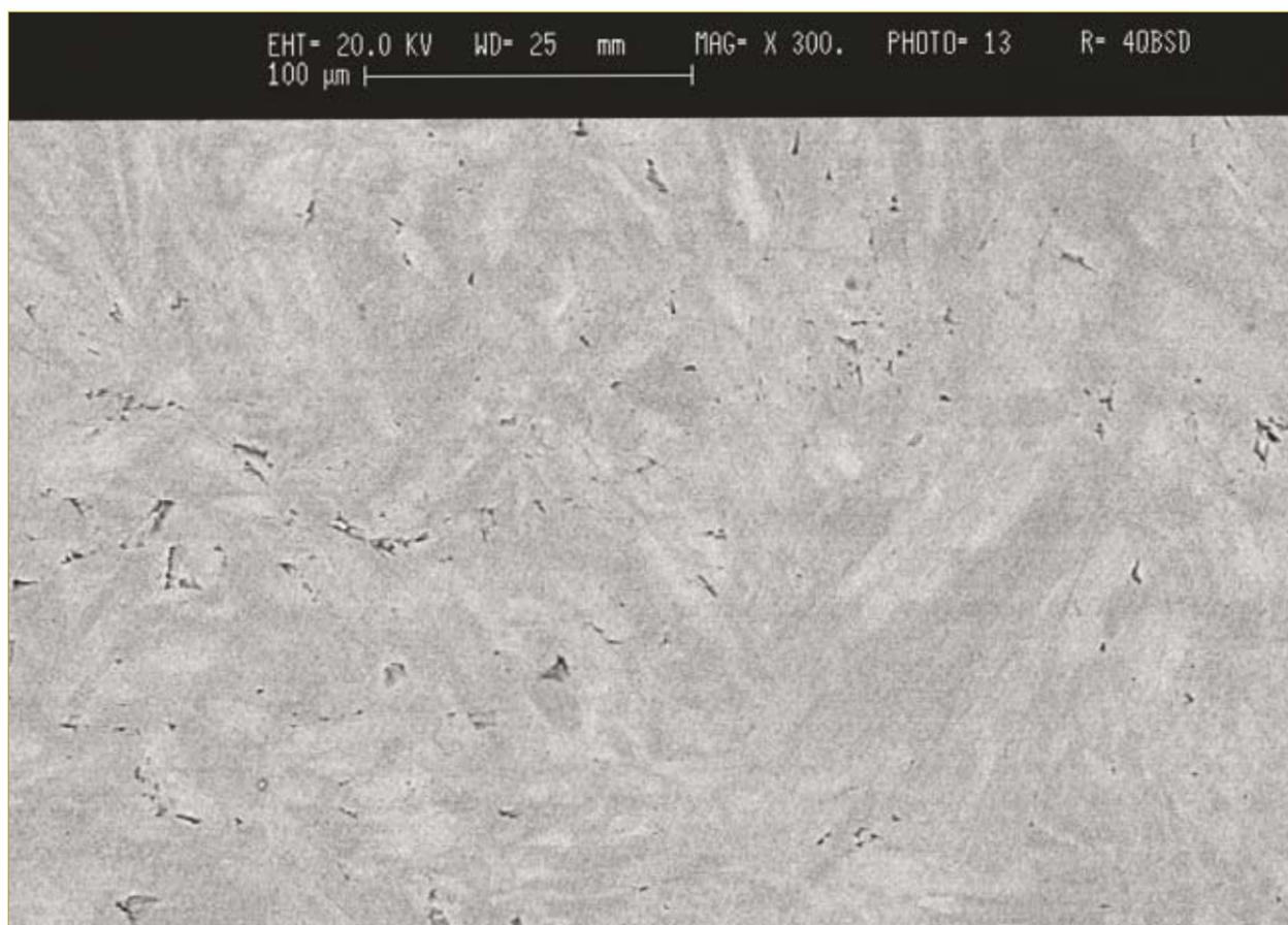
**Figure 3:** Back-scattered electron image of omphacite jade from the Po valley. The darker areas are richer in jadeite while the paler areas have higher contents of diopside-hedenbergite. Photo by Agostino Rizzi.
