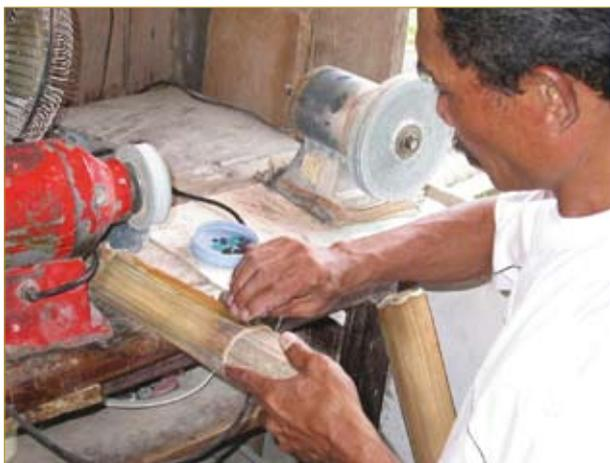
**Figure 6:** A local craftsman at Labuha, Bacan island, uses simple machinery for shaping and grinding of cabochons. Polishing with dry bamboo gives a very smooth surface to the stones.
