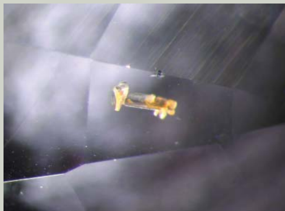
Figure 8: A cluster of brownish yellow platelets, probably mica, is an inclusion in a musgravite from Africa. Magnified 80x.
