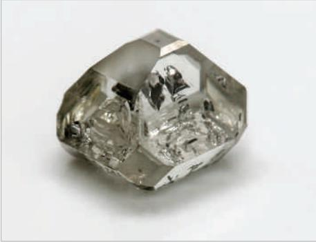
3: The classic crystalline habit of a HPHT-created diamond, this cubo-octahedron has octahedral and cubic faces. Also evident is the large metallic inclusion from the flux, which was used to help grow the synthetic diamond crystal.
