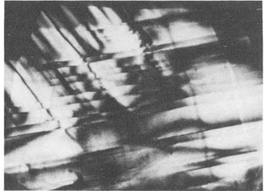
Fig. 10. Families of intersecting glide planes parallel to prism faces  $a$ ,  $a'$  and  $a''$   $\{1120\}$  in synthetic orange sapphire which was produced by the Verneuil technique; view in a direction parallel to the  $c$ -axis. Crossed polars 25 x.
