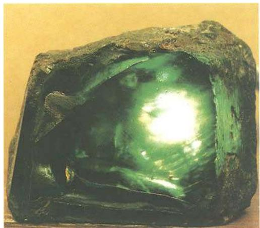
Fig. 4. A piece of metal (possibly aluminium) can be seen in the cavity in the top left-hand corner. Transmitted light.
