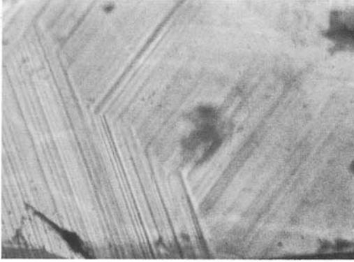
Fig. 9. Families of straight parallel growth planes that form an angle in natural ruby from Sri Lanka viewed in a direction parallel to the  $c$ -axis; planes parallel to prism faces  $a$  and  $a'$   $\{11\bar{2}0\}$  form an angle of  $120^\circ$ . 30 x.
