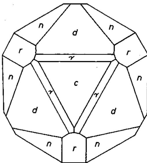
Fig. 3. Idealized single crystal of Chatham synthetic sapphire viewed in a direction parallel to the  $c$ -axis.
