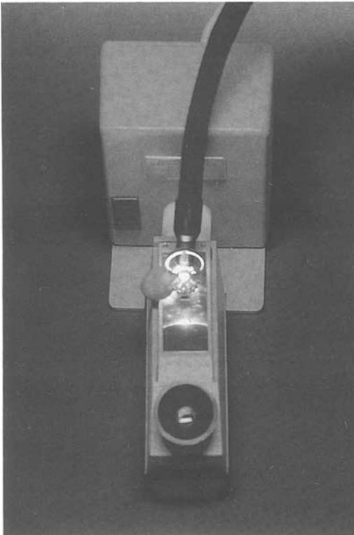
Fig. 2. Fibre optic light source directed on to the stone under test.
