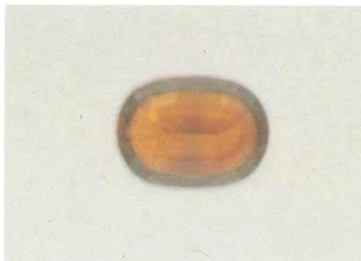
Fig. 4. The same stone from Fig. 3 is now shown just after it was exposed within 1 cm to the heat and light of a 150 watt spotlight for 15 minutes. The colour has become much darker and more brownish. After it returns to room temperature the colour will return to that in Fig. 3.
