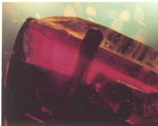
Fig. 4. Strong straight colour zones in the crown, and curved growth lines in the pavilion made visible when the stone is immersed in methylene iodide.
