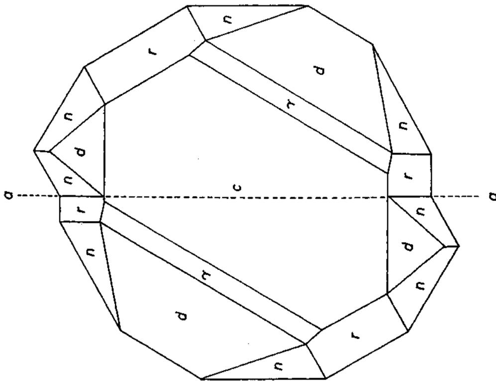
Fig. 4. Slightly distorted crystal of Chatham synthetic sapphire viewed in a direction parallel to the  $c$ -axis. The crystal reveals contact twinning across  $\{1010\}$  with  $a$   $\{1120\}$  as composition plane; re-entrant angles are formed by the faces  $n$  and  $r$ .
