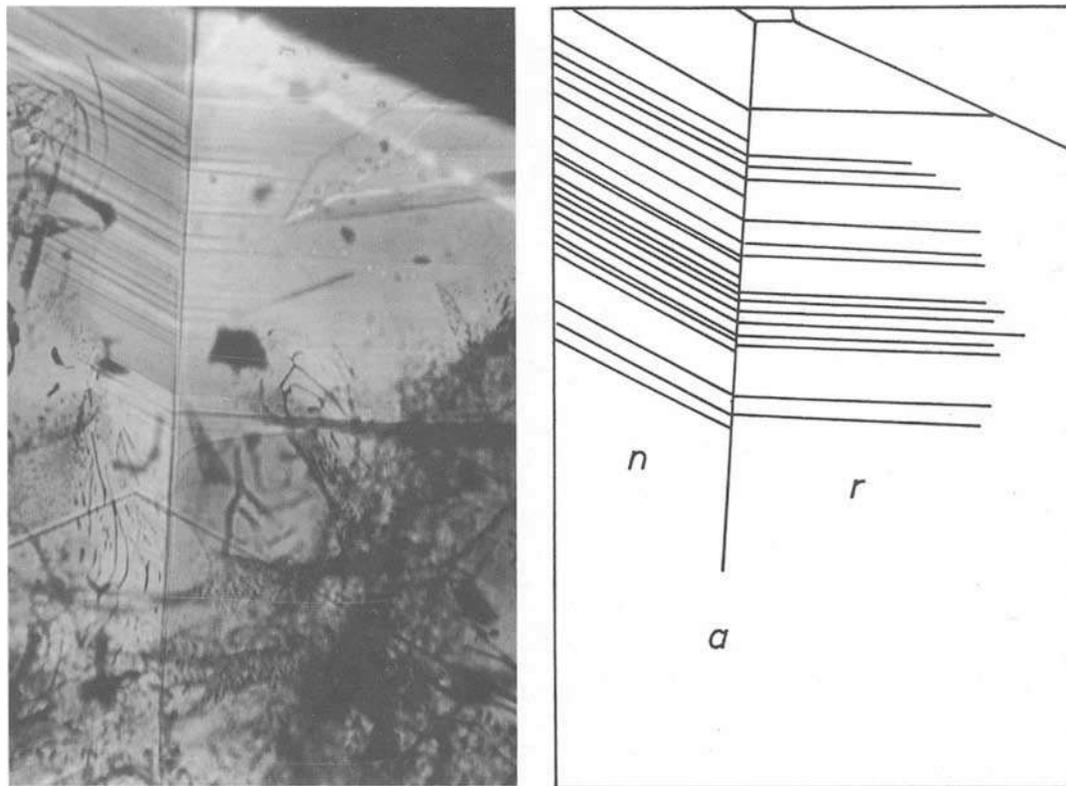
Fig. 7. Families of straight parallel growth planes in Chatham synthetic sapphire, growth sectors confined to the positive rhombohedron  $r$  ( $10\bar{1}1$ ) [right part] and the hexagonal dipyramid  $n$  ( $22\bar{4}3$ ) [left part] are divided by a twin boundary parallel to  $a$  ( $11\bar{2}0$ ); a re-entrant angle is formed by the faces  $n$  and  $r$ . Left: microphotograph, 40  $\times$ ; right: drawing of growth and composition planes.
