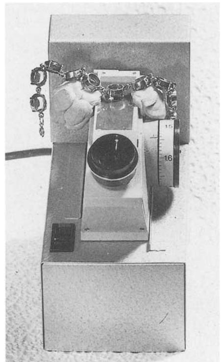
**Figs. 5 and 6.** Large balls of Blu-Tack are positioned on the flanks of the refractometer. These take a firm hold of the necklet and bracelet and allow them to be straddled across the prism so that one gem at a time may be carefully lowered into contact with the prism.
