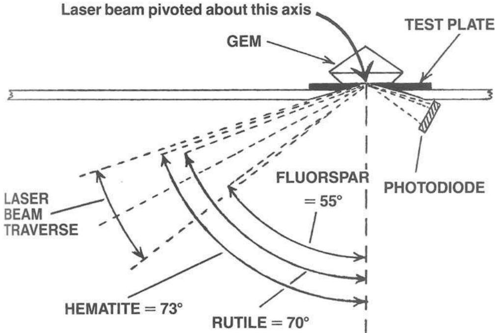
Fig. 5. Sketch showing the optics of the experimental refractometer.
