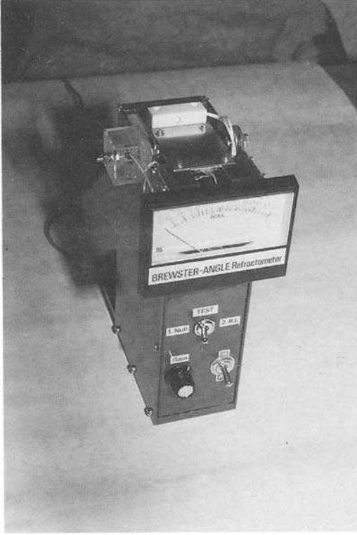
Fig. 3. (Left). View of the instrument's control panel. The panel meter is used via the two-position "TEST" switch for both null indication when pivoting the laser beam, and for direct readout of a gem's RI when the null is found.
