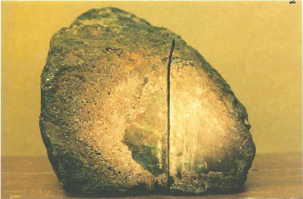
Fig. 2. The larger specimen cut in two. The surface has been scraped to show where the sand and pyrite had been stuck on.
