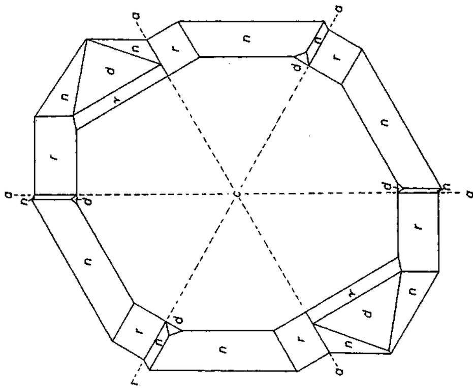
Fig. 5. Distorted crystal of Chatham synthetic sapphire viewed in a direction parallel to the  $c$ -axis. The crystal reveals repeated (cyclic) twinning across  $\{1010\}$  with  $a$   $\{1120\}$  as composition planes; re-entrant angles are formed by the faces  $n$  and  $r$ .
