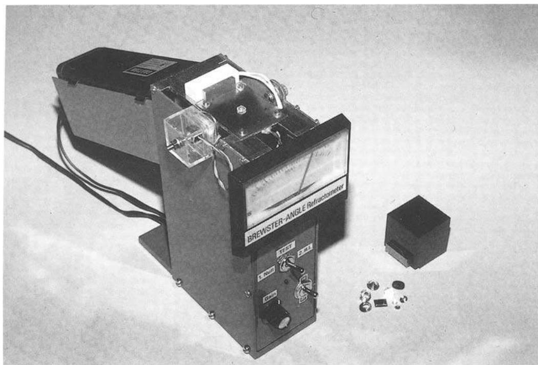
Fig. 2. General view of the experimental Brewster-angle refractometer. The magnetic interlock has been by-passed and the safety cover removed to show a synthetic rutile specimen illuminated by the laser beam.
