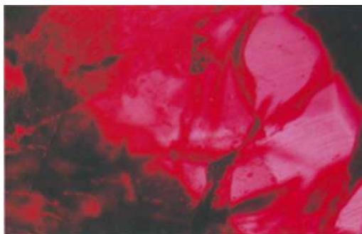
Fig. 10. Curved growth lines and the fractures, observed under the microscope in the synthetic Verneuil ruby.
