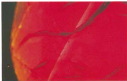
Fig. 9. Detailed view of a polysynthetic twin lamellae, observed under the microscope. Notice the fracture breaking the surface of the synthetic Verneuil ruby.
