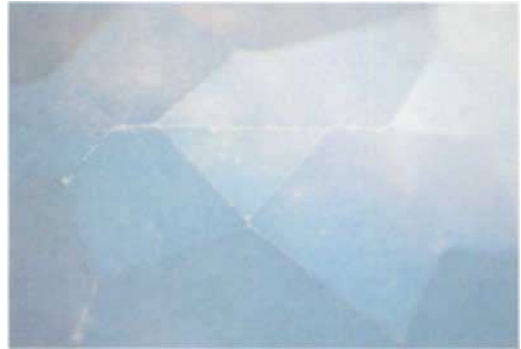
Fig. 7. The diagnostic white-appearing facet junctions on this treated topaz represent areas where either the treatment did not 'take' or where it has been abraded away. Magnified 10x. Diffused transmitted light. Photomicrograph by John I. Koivula, Gemological Institute of America.
