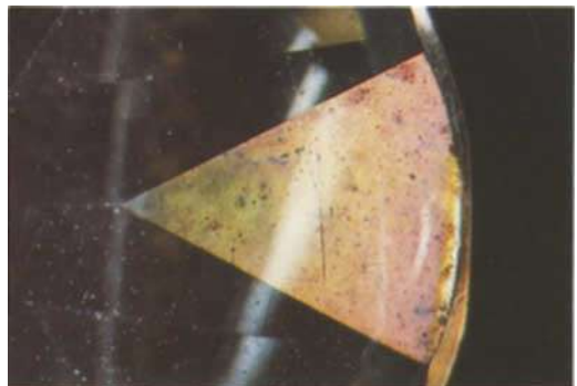
Fig. 10. When examined in surface-reflected light under magnification, the iridescence on this 'Aqua Aura' treated topaz becomes very noticeable and the surface irregularities are easy to detect. Magnified 12x. Photomicrograph by John I. Koivula, Gemological Institute of America.
