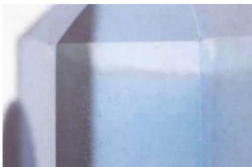
Fig. 4. Note the large colourless area on this treated quartz gem where there is no surface treatment Magnified 4x. Diffused transmitted light. Photomicrograph by John I. Kovula, Gemological Institute of America.
