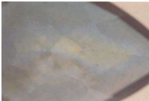
Fig. 9. Several of the facets on this treated topaz display irregular blue coloration. Magnified 6x. Diffused transmitted light. Photomicrograph by John I. Koivula, Gemological Institute of America.
