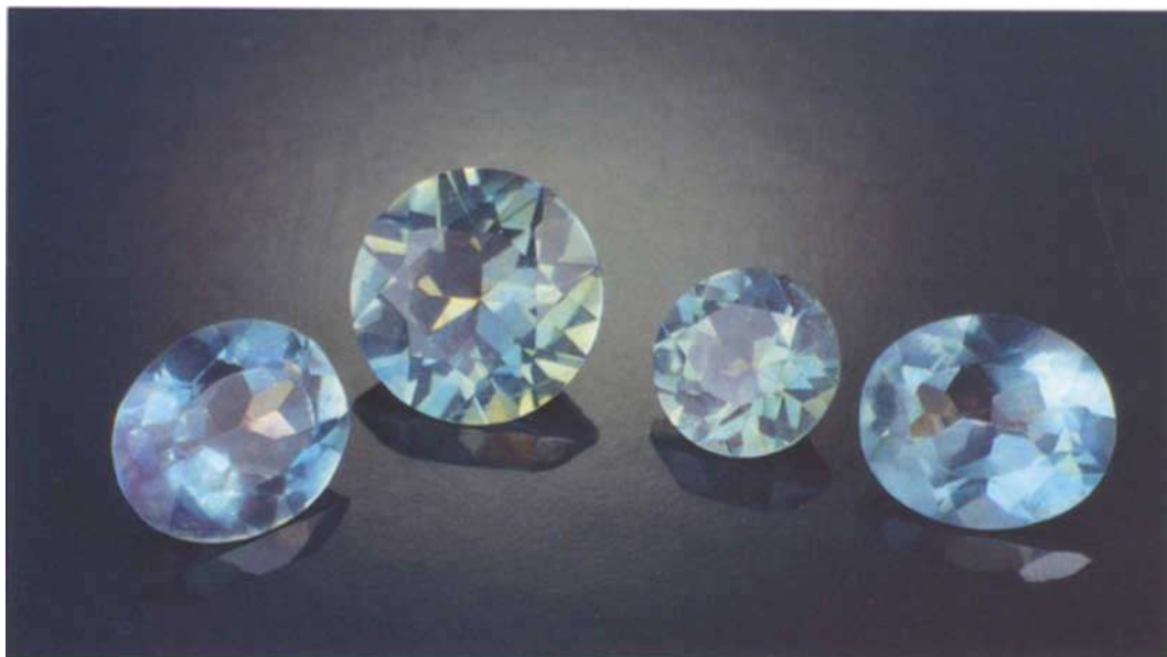
Fig. 2. These four faceted gems have all been treated by the 'Aqua Aura' process. The two in the centre are quartz, shown in their pre-treatment state in Figure 1; the two outer specimens are topaz. Photo by Robert Weldon, Gemmological Institute of America.
