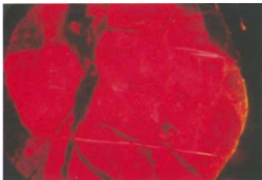
Fig. 8. Straight and parallel twinning striations as they appeared under the microscope, in the synthetic Verneuil ruby.
