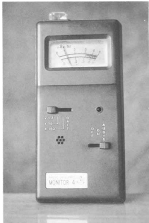
Fig. 4. The radioactivity of 0.12 mR/h recorded under the same conditions, but for the pair of glass imitation emeralds.
