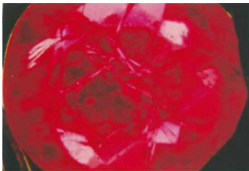
Fig. 5. Fractures and fingerprints as they appeared under the microscope, in the Verneuil synthetic ruby.
