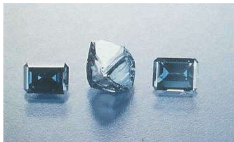
Figure 9: Originally near-colourless diamonds (0.33 ct, 1.15 ct and 0.36 ct) have been coated with a greyish-blue synthetic diamond film by A. Phelps at the University of Pennsylvania. Photo by R. Weldon, courtesy of GIA.
