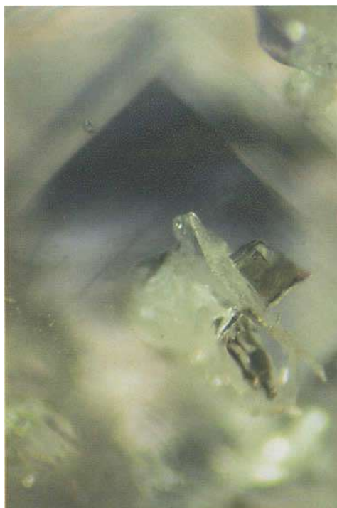
Figure 12: Sapphire, Andranondambo, Malagasy (Source A); a blue phantom containing a calcite fragment. 65x.
