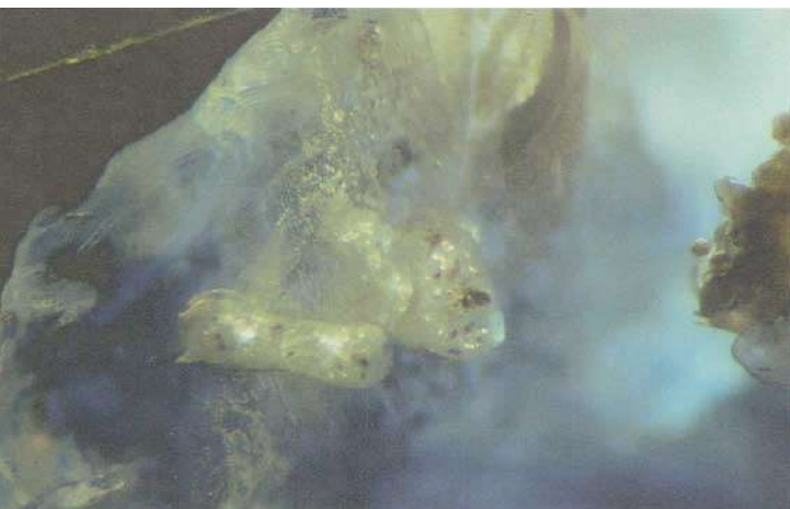
Figure 14a: Sapphire from Source A: two light calcite crystals beside botryoidal accumulation of F-phlogopite. 66x.
