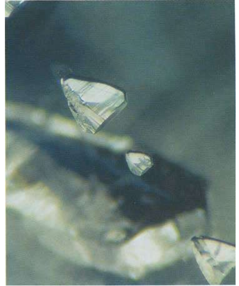
Figure 13b: Sapphire from Source A: negative dipyrramids n(2243) aligned along the c -axis, and blue colour phantom. 40x.
