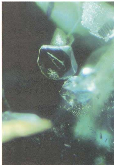
Figure 14a: Sapphire from Source A: two light calcite crystals beside botryoidal accumulation of F-phlogopite. 66x.
