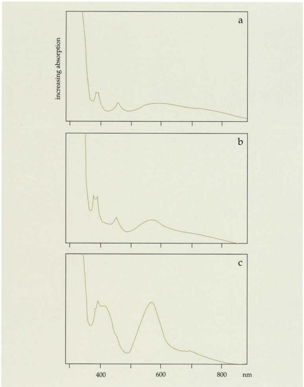
**Figure 15:** Absorption spectra of 'metamorphic' type fancy colour corundums from Barrington and West Pailin corundum suites.
