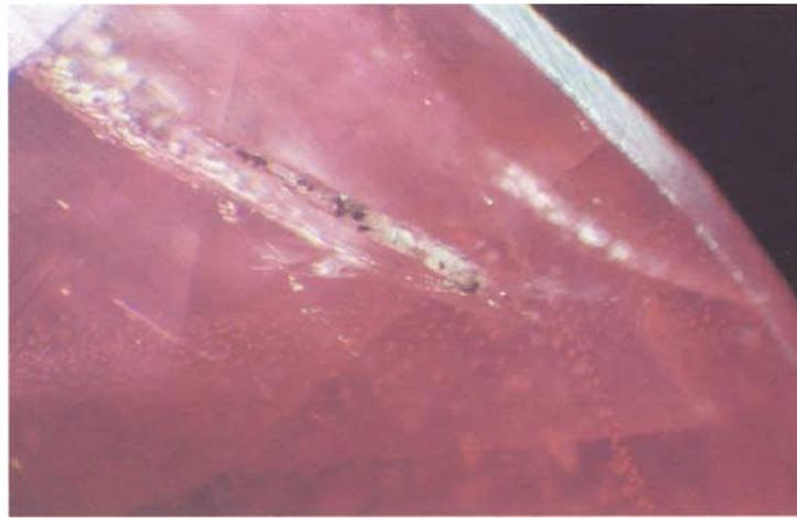
**Figure 6:** Oblong transparent, colourless crystals of plagioclase feldspar in a 0.80 ct purplish-pink sapphire from Pamir. Fibre-optic illumination, 48x.
