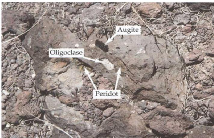
**Figure 8:** Typical specimen of the lava flow exhibiting single crystals of black augite, colourless (appears white) oligoclase feldspar and green peridot. Each crystal is approximately 5 x 2.5 x 2.5 cm.
