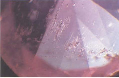
**Figure 5:** Calcite crystals, highly resorbed, in parallel rows form a distinctive inclusion pattern in the rubies and pink sapphires from Pamir. Fibre-optic illumination, 40x.
