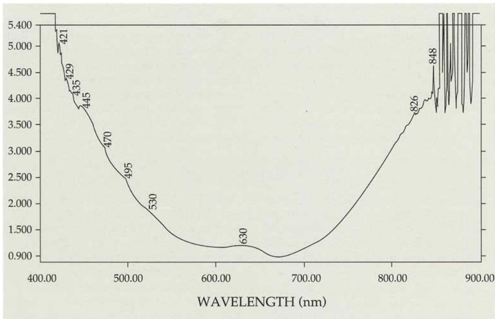
**Figure 14:** UV-visible spectrum of a representative sample of peridot from material found at Black Rock Summit lava flow – a 6.47 ct faceted stone (Figure 13, extreme left of picture) and recorded using a Pye-Unicam 8800 spectrophotometer.
