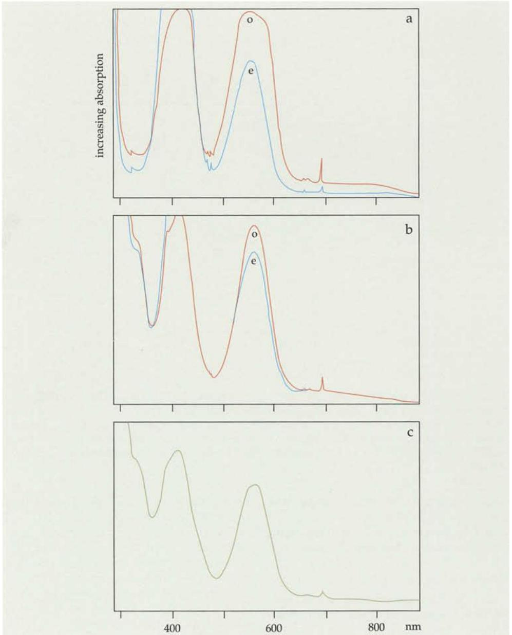
**Figure 13:** Comparative colour absorption spectra related to Cr-bearing corundums.
