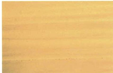
**Figure 21:** Countless dark orangy-brown near-parallel flow lines in transmitted light, possibly the result of exsolution. Photomicrograph by J. Koivula; 50x.
