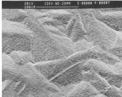
**Figure 6:** Scanning Electron Microscope photomicrograph, showing corroded surface of a pink corundum grain from Gloucester Tops, Barrington volcano. Note the strong etching leaving a criss-cross ridge-like surface morphology. Photograph by G. Avern and B.J. Barron, X100.
