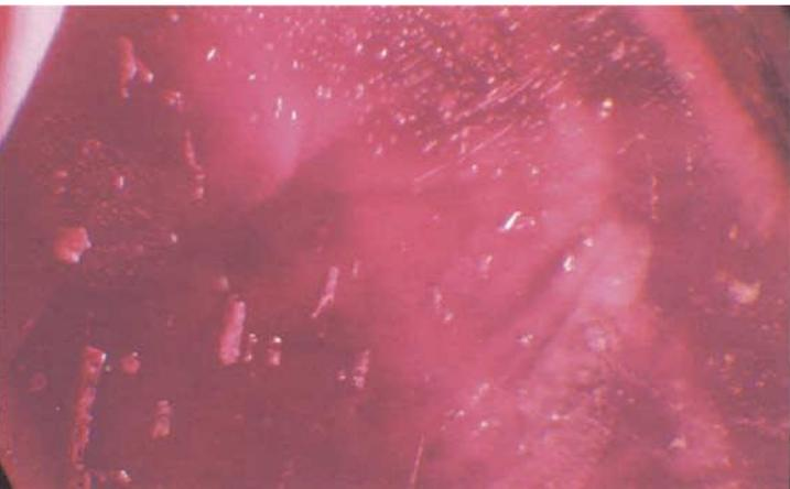
**Figure 8:** Idiomorphic negative crystals commonly contain immiscible liquid and gas phases. Fibre-optic illumination, 38x.
