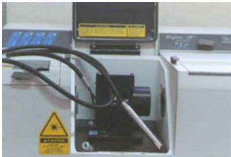
**Figure 1:** The near-IR fibre-optic probe accessory connected to the FTIR spectrometer.
