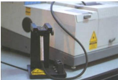
is connected with the stainless-steel probe and the other end is connected with the FTIR spectrometer by a special detector (Figure 1). White light (quartz-halogen) and a KBr beam-splitter were used. The wavenumber range scanned was from  $6500$  to  $4200\text{ cm}^{-1}$  with a resolution of  $8\text{ cm}^{-1}$ ; the scan number was 10.
