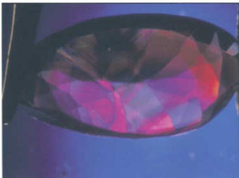
*Figure 9b: The piece shown in Figure 9a is observed under cross polarised light. The yellow area clearly shows Brazil twinning.*
