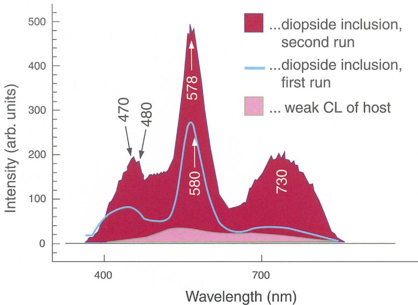
**Figure 18:** The CL spectra of the colourless diopside inclusion shows a diagnostic band at 578 nm. The different intensities between the first and the second run reflect the CL colour change of the inclusion from yellowish-white to pale red during longer bombardment. Excitation conditions: 9.0 kV; 0.8 mA.
