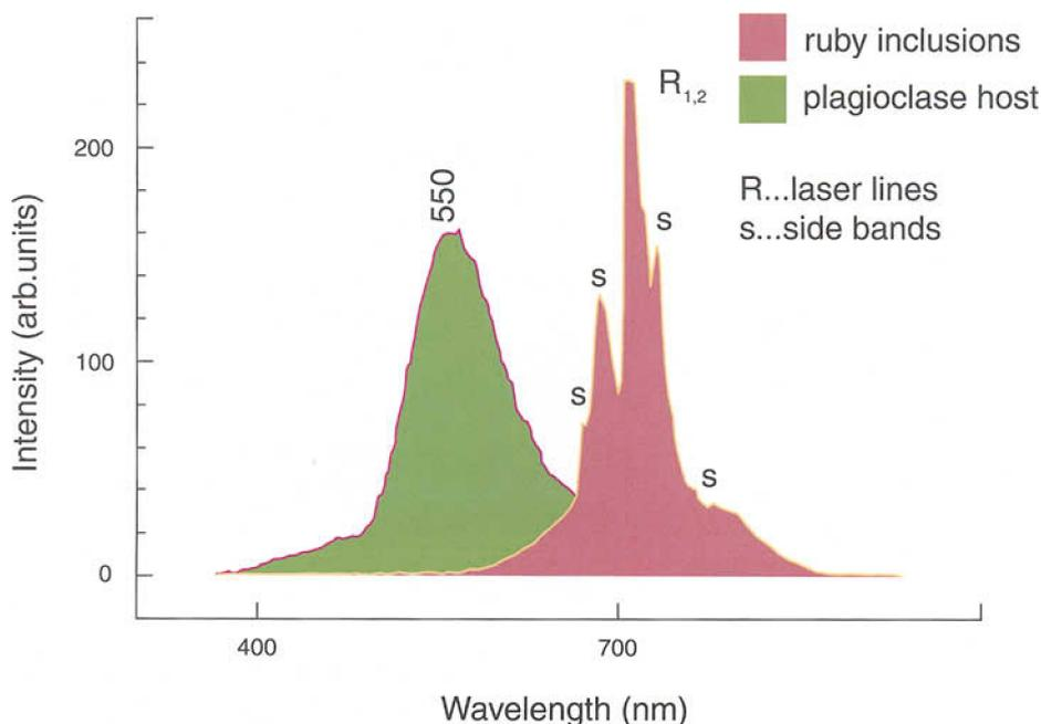
**Figure 22:** CL spectra of the plagioclase host and ruby inclusions. Excitation conditions: 5.0 kV; 0.4 mA
