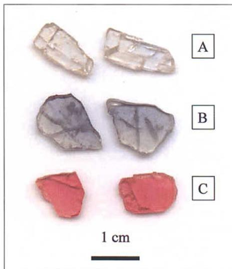
**Figure 2:** Polished slices of Chimwadzulu corundum.
