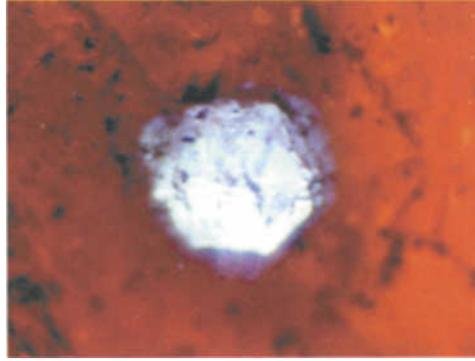
Figure 23: Red CL of a greyish-blue rough calcite with two whitish luminescing dots of albite. Excitation conditions: 9 kV; 0.9 mA. Enlargement: 10 x.
