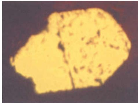
**Figure 10:** The yellow luminescent apatite at higher magnification. The colour is caused by  $Mn^{2+}$ ,  $Dy^{3+}$ ,  $Sm^{3+}$  and  $Sm^{2+}$  ions replacing  $Ca^{2+}$  ions in the apatite structure. Excitation conditions: 15 kV; 0.95 mA. Enlargement: 125 x.
