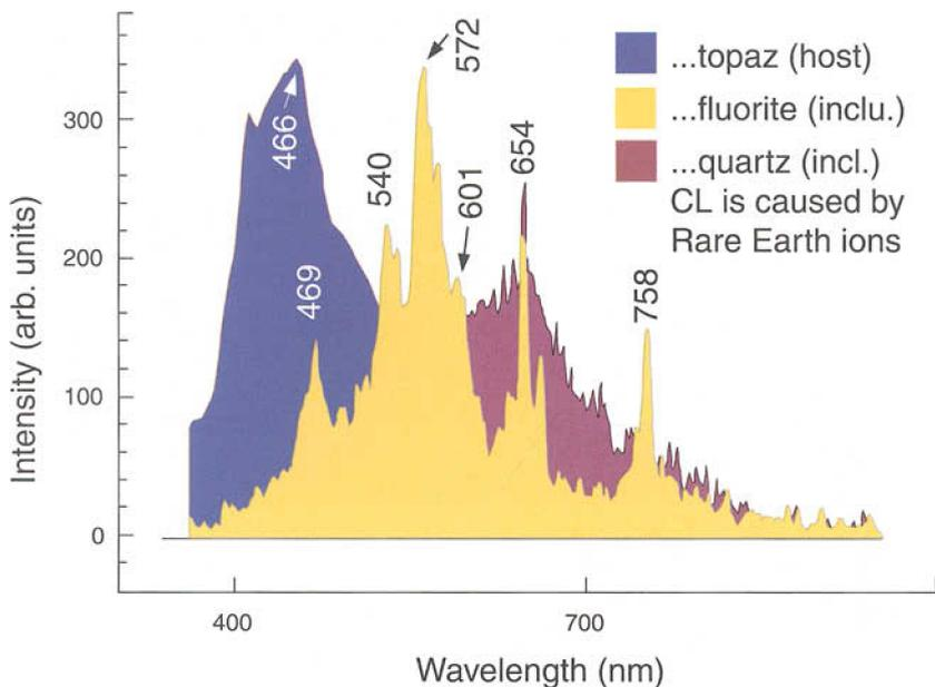
**Figure 8:** CL spectra of host and inclusions. Topaz is shaded blue (dark maroon in Figure 7), quartz is shaded violet, and fluorite yellow. Excitation conditions 12.5 kV; 0.9 mA.
