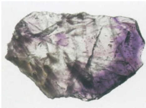
**Figure 4:** The rough stone shown in Figure 2 was cut along the direction of the *c*-axis. The top end of the piece shows intense purple.
