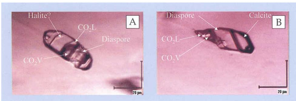
**Figure 8:** Multiphase CO<sub>2</sub>-diaspore inclusions in gem ruby. Both CO<sub>2</sub> liquid and vapour are visible at room temperature (c. 20°C). (A) The inclusion also contains a cubic daughter phase believed to be halite. (B) The inclusion also contains calcite confirmed by LRM (see Figure 9).
