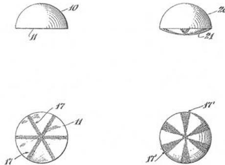
**Figure 1:** By scratching the flat (left) or curved (right) surface of a cabochon-cut gemstone in different regions, asterism is produced which can be seen as a moving star from various directions relative to a light source; 10, 20 cabochon-cut gemstones, 11 flat base of the gemstone, 21 curved surface of the gemstone, 17, 17' engraved areas with artificially produced scratches or grooves (from Mukai, 1950).
