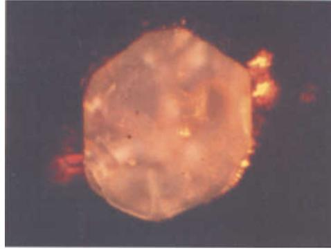
Figure 19: Brownish-yellow CL of a euhedral apatite in a non-luminescing kornerupine host. Excitation conditions: 9.0 kV; 0.9 mA. Enlargement: 125  $\times$ .
