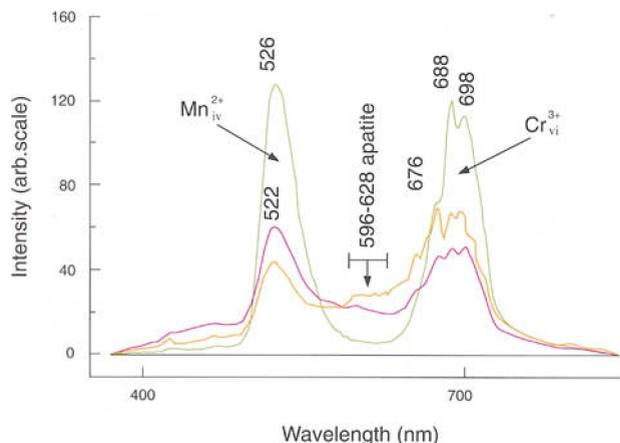
**Figure 4:** CL spectra of the host spinel with two distinct bands. The shorter wavelength one is caused by  $Mn^{2+}$  ions in tetrahedral configuration, the other by  $Cr^{3+}$  ions in octahedral configuration. The shoulder between both bands can be ascribed to  $Mn^{2+}$  ions of the apatite inclusion, sevenfold co-ordinated.
