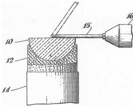
**Figure 2:** Production of scratches on the flat base of a cabochon-cut gemstone by use of a rotating or vibrating iron rod; for the artificial production of scratches or grooves on curved surfaces, the rod is held at an angle to the surface (dot and dash lines); 10 cabochon-cut gemstone, 12 cement, 14 support, 15 iron rod, 16 rotating chuck (from Mukai, 1950).
