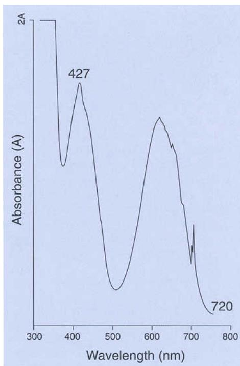
**Figure 4:** The UV/Visible spectrum for a Gilson N-type flux-melt synthetic emerald displaying the 427 nm absorption band.
