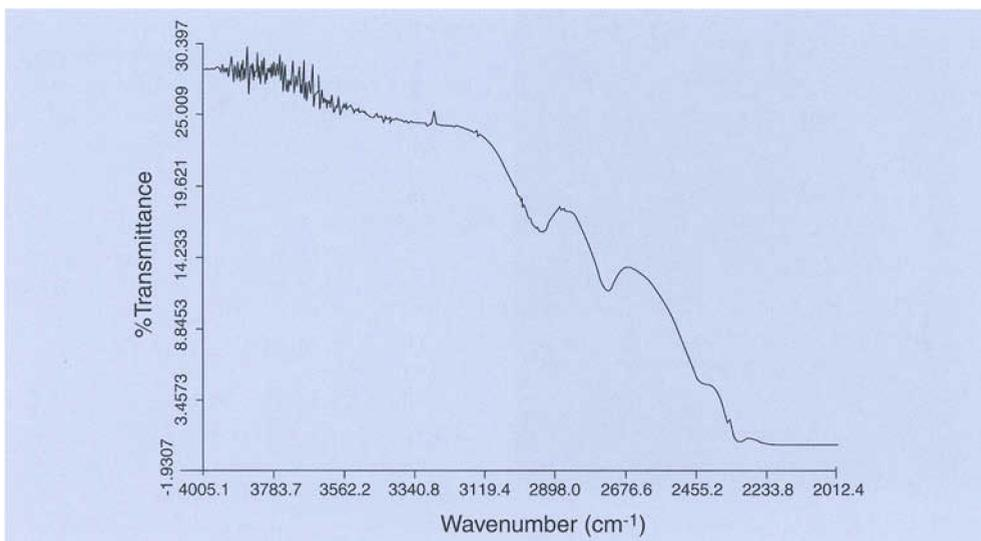
**Figure 3:** FTIR spectrum of the Gilson N-type flux-melt synthetic emerald showing the lack of absorption between  $3400\text{ cm}^{-1}$  and  $4000\text{ cm}^{-1}$ .
