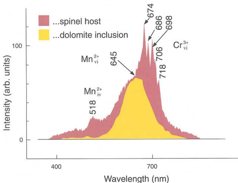
**Figure 6:** CL spectra of the spinel host (pink) and curve-fitted dolomite spectrum (orange). Excitation conditions: same as in Figure 5.
