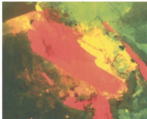
**Figure 21:** The bright red luminescence of ruby inclusions provides a perfect contrast to the green CL colour of the plagioclase host. The CL colour of the latter is evoked by  $\text{Mn}^{2+}$  ions. The dark areas on the left are pargasite and the small black blotches are caused by picotite grains. Excitation conditions: 10.5 kV; 0.8 mA. Enlargement: 40 x.
