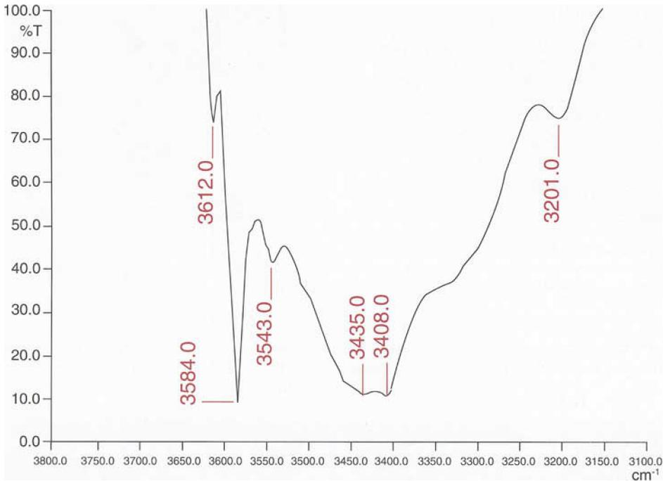
**Figure 12:** The infrared absorption spectrum of a natural amethyst from the Caxarai mine. Absorption at  $3543\text{ cm}^{-1}$  is clearly seen.
