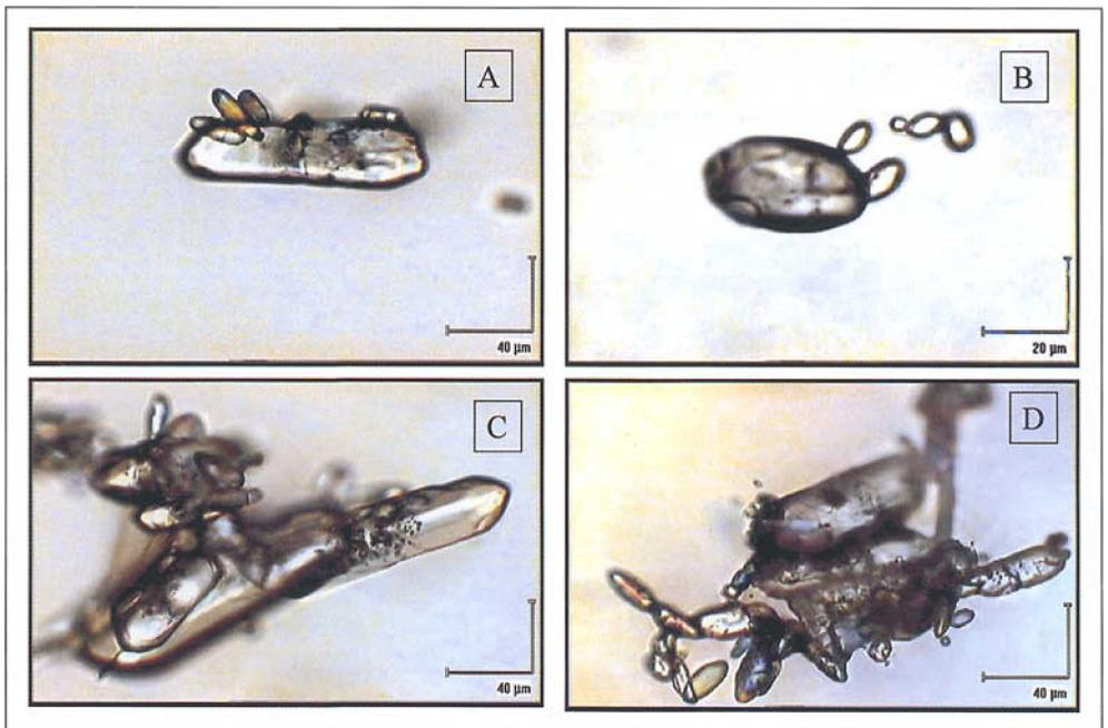
**Figure 3:** Zircon clusters in colourless corundums (partially crossed polars). Scale bar represents 40  $\mu\text{m}$  for A, C and D, and 20  $\mu\text{m}$  for B.
