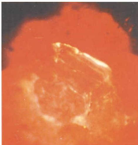
**Figure 5:** Yellow CL of a euhedral dolomite crystal inclusion at the surface of the spinel. Part of the inclusion and tension haloes are very near to the surface of the host as yellow luminescing clouds. Excitation conditions: 16 kV; 0.8 mA. Enlargement: 100 x.
