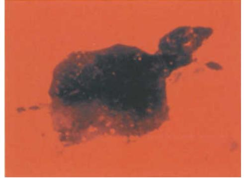
**Figure 13:** Red CL of the host crystal with an inert rutile inclusion. It exhibits a strong broad CL band in the NIR. Excitation conditions: 11.0 kV; 0.9 mA. Enlargement: 40 x.
