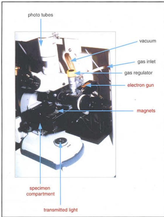
**Figure 2:** The 'cold-cathode' unit with the electron gun flanged to the compartment rests on the table stand of a binocular microscope. For microspectrophotometry the whole assemblage is set in a frame on which the motor-driven monochromator and photomultiplier is mounted. Vacuum pump, amplifier and computer are not shown.
