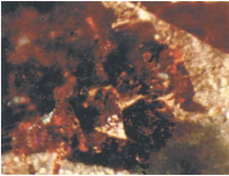
**Figure 12:** Rutile inclusions in kyanite at the surface of a pavilion facet. Incandescent light, stereomicroscope ZEISS STEMI 2000C.
