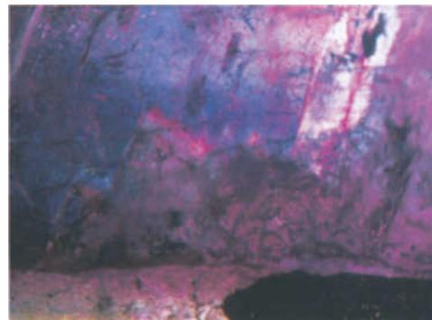
**Figure 6b:** The same piece in Figure 6a is observed under cross polarised light. The *z* sector displays a uniform interference colour of violet, indicating that the area has no Brazil twinning.
