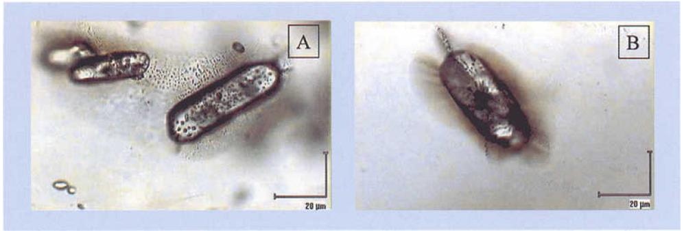
**Figure 5:** Zircon inclusions in heat-treated corundum with characteristic dark outlines, 'feathers' and trails of secondary inclusions in discontinuous fractures associated with each zircon. Scale bar represents 20  $\mu\text{m}$ .
