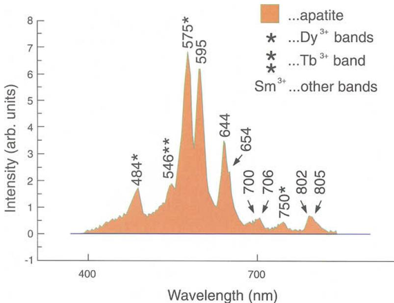
Figure 20: CL spectrum of a brownish-yellow luminescing apatite inclusion in a green kornerupine from Sri Lanka exhibiting narrow REE<sup>3+</sup> bands caused by trivalent dysprosium, terbium and samarium. Excitation conditions: 9.0kV, 0.9 mA.
