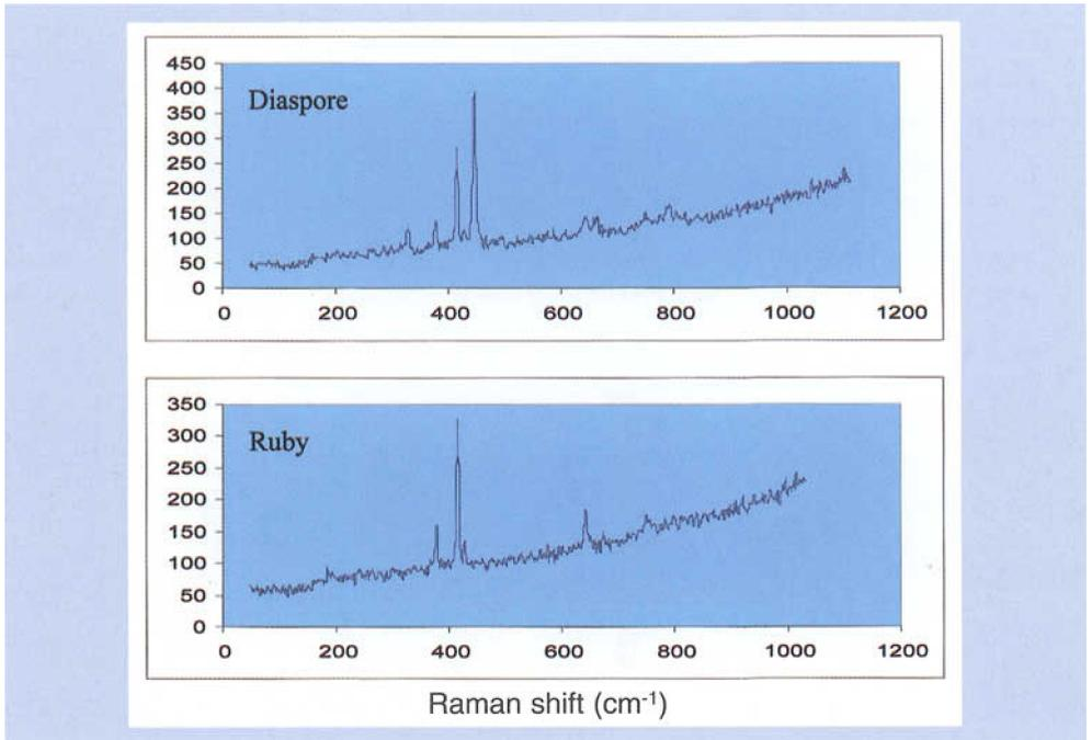
**Figure 6:** Raman spectrum of a single crystal of diaspore from unheated, colourless, Chimwadzulu corundum. Spectrum of ruby shown below for comparison.
