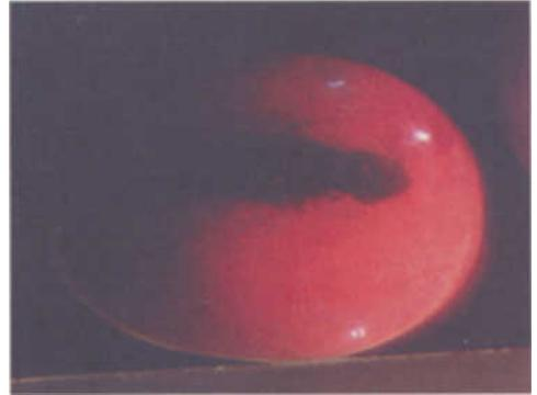
**Figure 27:** Dolomite under electron bombardment shows up in a violet-tinted red, the pargasite remains inert. Excitation conditions: 9 kV; 0.8 mA.
