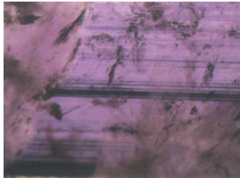
**Figure 5:** A piece of Caxarai amethyst sliced perpendicular to the *c*-axis is observed along the direction of the *z* {0111} face. Extremely sharp colour zoning is present.
