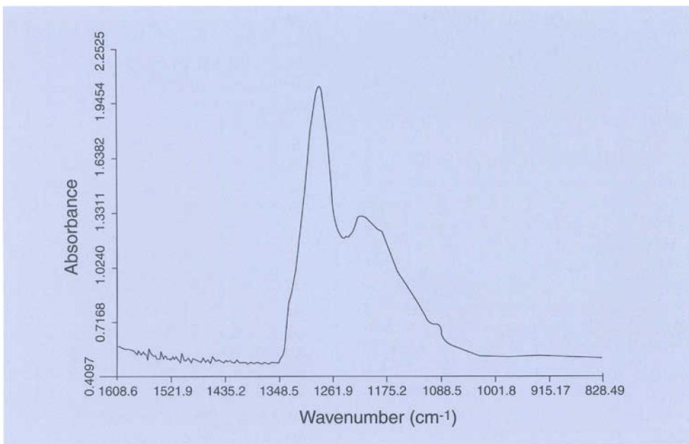
**Figure 6:** The FTIR spectrum of the 0.34 ct yellow synthetic diamond. The main peak at  $1282\text{ cm}^{-1}$  categorizes the diamond as type IaA (pairs of nitrogen atoms). The shoulder on the left-hand side of the peak is in the general area of the  $1344\text{ cm}^{-1}$  peak, which indicates a small amount of type Ib (single nitrogen atoms).
