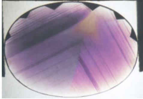
*Figure 8: The colour zoning in two directions parallel to the z face.*
