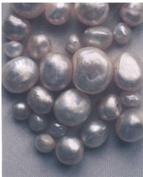
**Figure 7:** Partly coated natural pearls. The grainy surface of the applied coating can be observed next to the platy nacreous surface.
