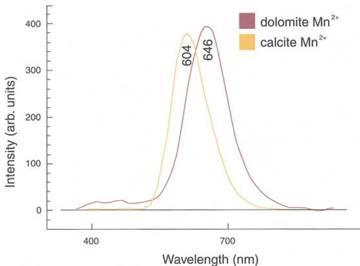
**Figure 28:** CL spectra of dolomite and calcite hosts, the first used as a simulant of jade (Figure 26). In both minerals CL is provoked by manganese ions. Calcite shows a more orange to brick-red CL colour, whereas dolomite luminesces violet-tinted red. The main peak of the latter is shifted into the red by more than 40 nm.
