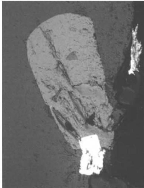
**Figure 16:** SEM photo of the diopside inclusion in a green tourmaline (dark grey) with an adhering zircon crystal (white). Compare also the X-ray diagram of Figure 17.
