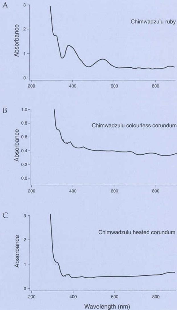
**Figure 1:** Absorption spectra (unpolarized) of Chimwadzulu corundums.
