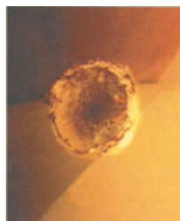
**Figure 3:** CL of a globular apatite inclusion showing an orange CL colour. Its true colour is masked by the strong CL of the host crystal. Excitation conditions: 12 kV; 0.85 mA. Enlargement: 40 x.
