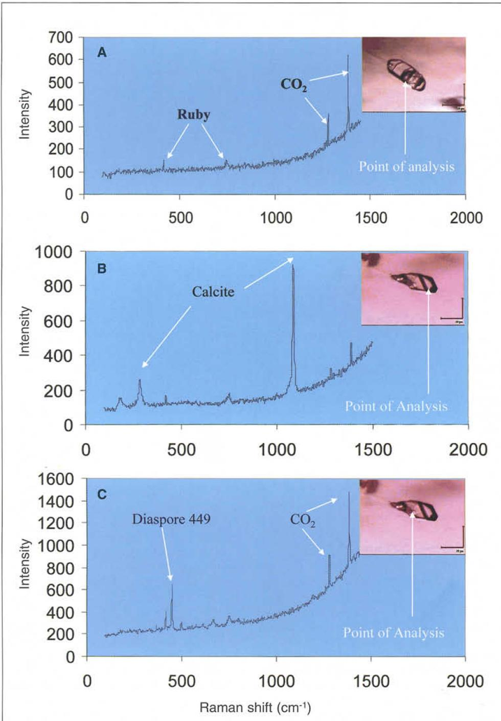
**Figure 9:** Raman spectra of diaspore, CO<sub>2</sub> and calcite of inclusions shown in Figure 8 above. (A) CO<sub>2</sub>-rich phase: note also peaks from the host ruby. (B) Calcite; note weaker 'interference' peaks from CO<sub>2</sub> and ruby. (C) Diaspore; note 'interference' peaks from CO<sub>2</sub> and ruby.
