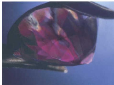
**Figure 11b:** The same piece in Figure 11a is seen under cross polarised light. The Brazil twinning is present in the r sector.
