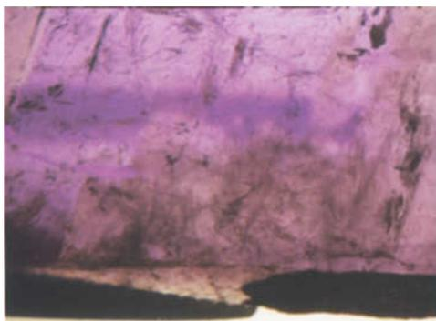
**Figure 6a:** A piece of Caxarai amethyst sliced perpendicular to the *c*-axis is observed along the optic-axis direction. The *z* sector appears dark purple.
