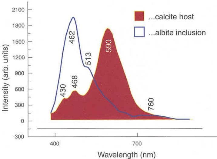
Figure 25: CL spectra of the rough calcite that hosts two albite inclusions. The host spectrum is dominated by a  $Mn^{2+}$ -band at 590 nm characteristic for the CL of calcites. The albite inclusion shows a strong band in the violet-blue with its tail reaching into the NIR. This band shape is indicative for defect centres causing the blue CL of the albite inclusion. The intensity of the calcite spectrum is multiplied by a factor of 10.
