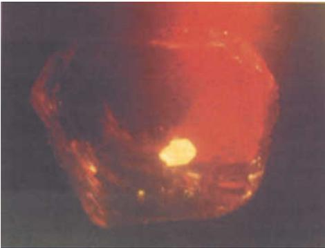
**Figure 9:** An orange umbralite with an apatite inclusion. The luminescing quartz inclusion is not visible. Excitation conditions: 15 kV; 0.95 mA. Enlargement: 40 x.
