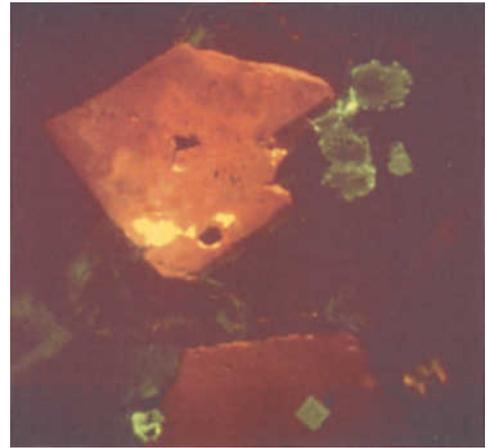
**Figure 7:** Reddish-brown CL of quartz and green CL of fluorite inclusions both activated by rare earth elements. Steel-blue CL colour of the host (to the eye) has turned into dark maroon in the photomicrograph. Enlargement: 125 x. Excitation conditions: 12.5 kV; 0.9 mA.
