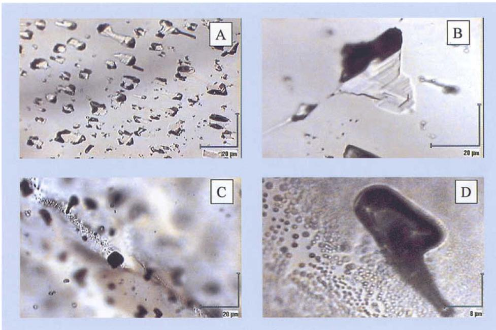
**Figure 7:** (A) Planar grouping of pseudosecondary, diaspore-CO<sub>2</sub> inclusions in colourless corundum. (B). Close-up of one of the inclusions in (A) showing a large diaspore crystal (lighter area) and a CO<sub>2</sub>-rich phase (dark area). (C) and (D) Dark 'empty' inclusions in heat-treated corundum with associated trails of smaller, empty inclusions in microfractures. Scale bar for A, B, C: 20 µm. Scale bar for D: 8 µm.
