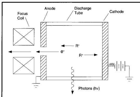
*Figure 1: Schematic diagram of a cold cathode electron gun. Discharge tube, focus coil and compartment are flanged together and filled with a carrier gas at a low pressure. (Reproduced from Marshall, 1993.)*
