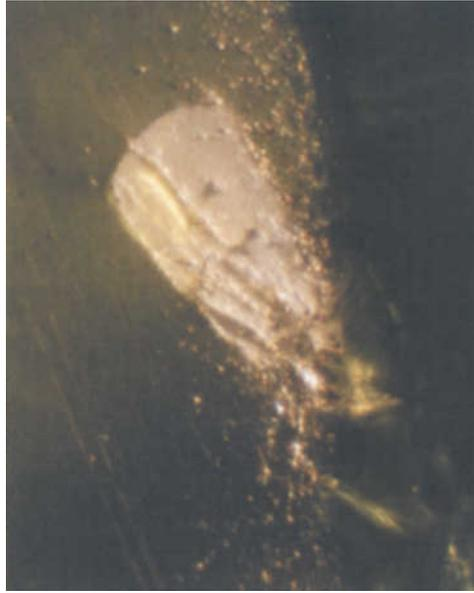
**Figure 15:** Pale red CL of a colourless diopside inclusion in a green non-luminescent tourmaline, Langenai, Tanzania. Excitation conditions: 0.8 mA; 11.0 kV. Enlargement: 125 x.
