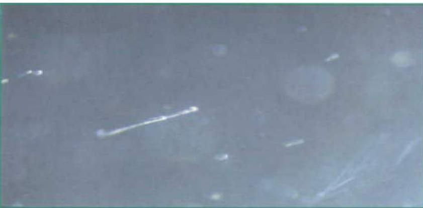
Figure 2: Needle-like structures form a characteristic inclusion pattern in the musgravite pebble. Magnified  $200 \times$ .
