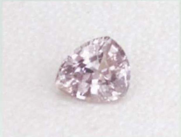
**Figure 3 (Specimen C):** This faceted taaffeite of 0.30 ct, size  $3.9 \times 4.6 \times 2.6$  mm, is a high zinc-bearing taaffeite from Sri Lanka.
