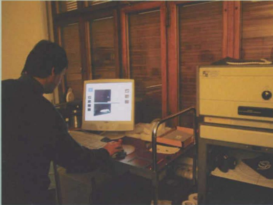
*Figure 1: Working situation with X-ray apparatus, CCD camera and screen. A pearl necklace is ready in the X-ray chamber, the camera F-View II is visible. Photo H.A. Hänni © SSEF Swiss Gemmological Institute.*
