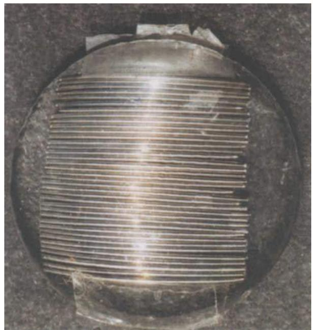
Figure 4: Cat's-eye effect produced by pins taped to the flat underside of a plano-convex lens.
