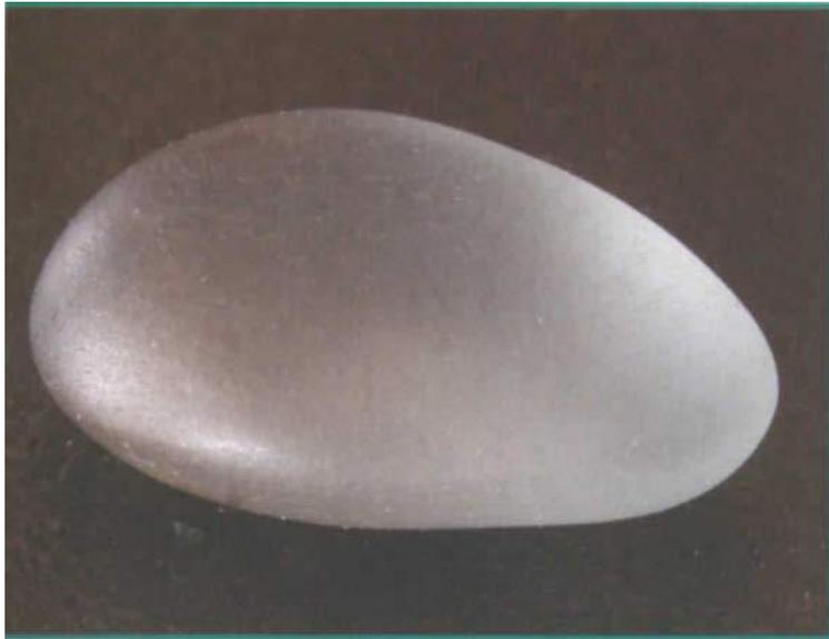
Figure 1: This water-worn pebble of 1.42 ct, size about  $8.4 \times 5.5$  mm, represents the first rough gem-quality musgravite found in Sri Lanka.
