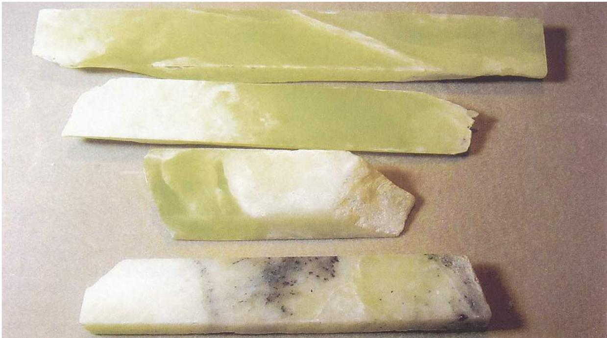
*Figure 6: Slab specimens of nephrite jade from Mastabia. Slab size approximately 10 mm wide. Foreground specimen contains inclusions of opaque iron minerals. Photo by Herbert Giess.*
