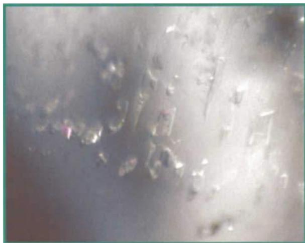
Figure 6: Negative crystals with multiphase fillings in zinc-rich taaffeite of 0.30 ct from Sri Lanka; magnification 100 ×.
