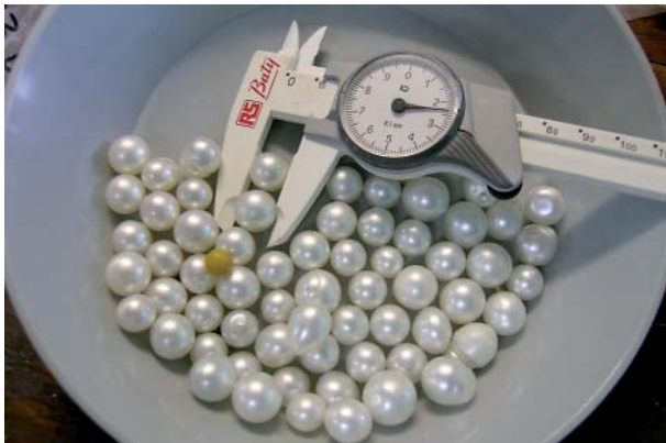
Figure 11: A small trial harvest provides data on the present quality of the pearl surfaces. The picture shows a bead (yellow, width 6.5 mm) in comparison with pearls produced after 18 months in the shell. The mean diameter is about 12.5 mm. Photo © H.A.Hänni.
