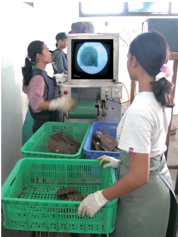
Figure 4: X-ray monitoring after a cleaning process shows whether the bead has been retained in the oyster. Photo © H.A. Hänni
