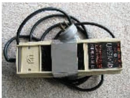
Figure 2: A combined LW and SWUV lamp UVSL-15 from UltraViolet Products (UVP).
