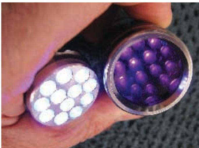
Figure 12: Multiple-LED torch of Figure 10 on the right next to a multiple-LED torch on the left which is unfiltered and emits light at and around 405 nm.
