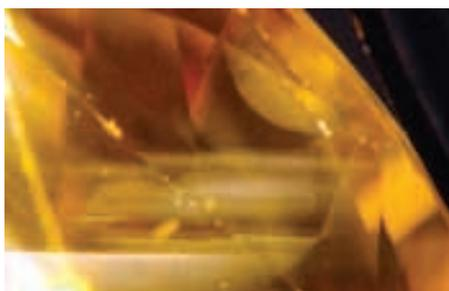
Figure 2: Broad parallel straight growth zonal striae lying in different planes and crossing each other at angles. Dark field illumination, magnification 15x.
