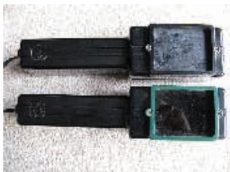
Figure 1: Separate LWUV and SWUV lamps manufactured by the Gemmological Association of All Japan (GAAJ).
