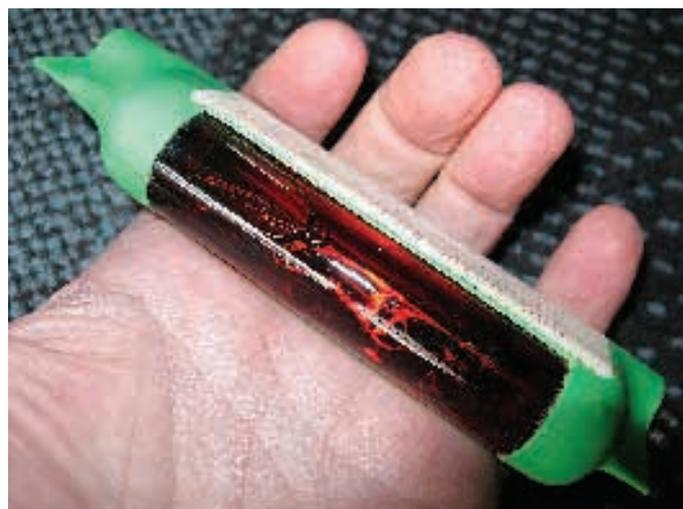
Figure 16: Small BLB 'black light' fluorescent LWUV tube (4 watt) above a 'germicidal' SWUV mercury based (4 watt) fluorescent tube fitted with a  $\text{CoSO}_4$  solution filter and green sleeve.
