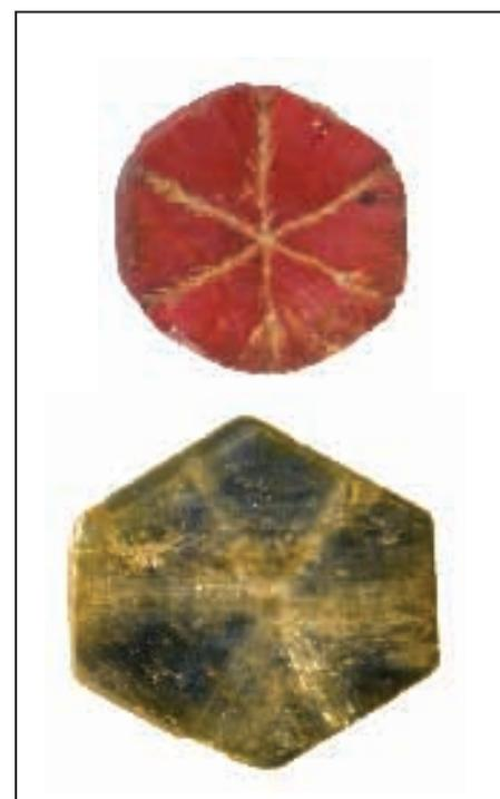
Figure 22: Trapiche ruby from Mong Hsu, Myanmar (top) and trapiche-type sapphire from Hunan province, China (bottom); slices perpendicular to the *c*-axis, the hexagonal outlines of the rough crystals are represented by dipyrnidal faces. With identical crystallographic orientation of both corundum slices, the different orientation of the fixed star within these samples is observed. Diameter of the trapiche ruby 4.20 mm, size of the trapiche-type sapphire 10 × 12 mm. Photos by K. Schmetzer.
