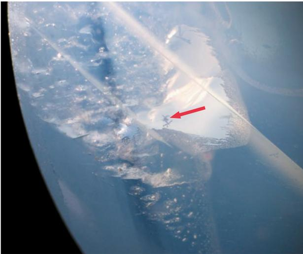
**Figure 10:** Magnification reveals twin planes and a healing fissure with dotted fluid inclusions in the Roman sapphire intaglio. The larger fluid inclusions show structured expansion discs. The main expansion disc contains tiny, radially arranged needles (see arrow) interpreted as Al-hydroxide precipitates. Photomicrograph by M. S. Krzemnicki, SSEF; image width 3 mm.
