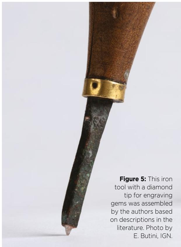
**Figure 5:** This iron tool with a diamond tip for engraving gems was assembled by the authors based on descriptions in the literature. Photo by E. Butini, IGN.
