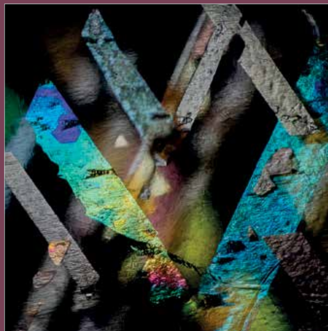
Ilmenite and hematite in orthoclase feldspar from Harts Range, Australia. Field of view 3.05 mm.
