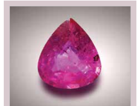
This 1.75 ct pear-shaped stone proved to consist of a sapphire doublet containing fissures and cavities filled with lead glass. Photo by S. Saengbuanglam.
