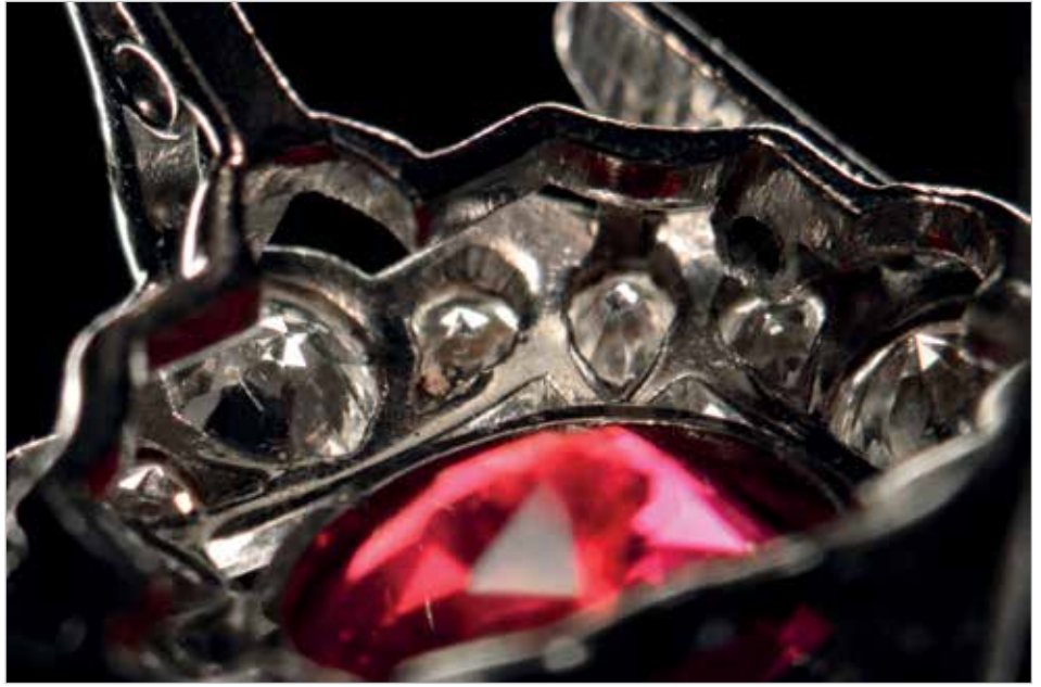
18: The holes for the small diamonds are shaped and the whole back is polished. Magnification approx. 12x.
