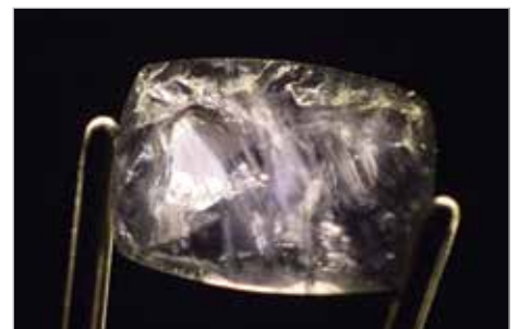
Fractures and wispy linear aggregates of microcrystalline chloritoid and/or chlorite form conspicuous inclusions in these sekaninaite gemstones (left magnified 5× and right 3×). The stone on the left also contains ferrogdrite (see arrow). Photomicrographs by R. Hanus.
