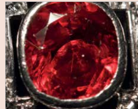
5: Centre stone (a) displaying fracture plane, top lighting (the white spot is a cavity in the table) and (b) seen from below, displaying fracture plane and surface cavity. Magnification approx. (a) 12× and (b) 8×.
