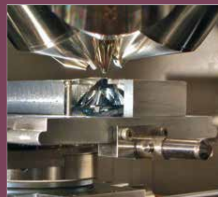
The Hope diamond in the Time-of-Flight-SIMS instrument. Photo Jeffrey Post.
