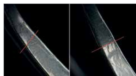
16: Inside the ring shank can be seen a polished finish above the red line with a dimpled surface below, due to being hammered on a triblet.
