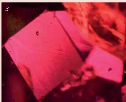
3: Isolated crystals (the one on the right with double image under two facets) and colour swirls. Magnification approx. 40×.
