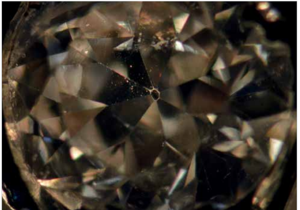
22: The lower pavilion facets reach about halfway to the small culet. Magnification approx. 40×.
