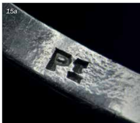
15: (a) Punch mark and (b) stock-reference punch mark inside shank.
