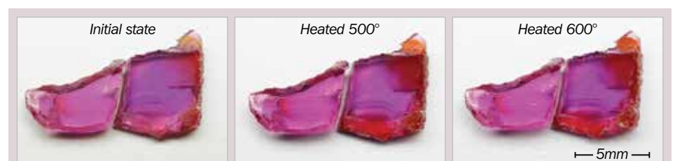
The iron-stained fractures in this representative sample of Mozambique ruby display a noticeable increase in orangey red coloration in the heated half (right side) compared to the untreated portion (left side). Photos by Y. Lhongsomboon.
