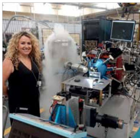
2: Sarah Steele and the small particle accelerator. The gamma-ray detector is cooled to -200^{\circ}\text{C} using liquid air.
