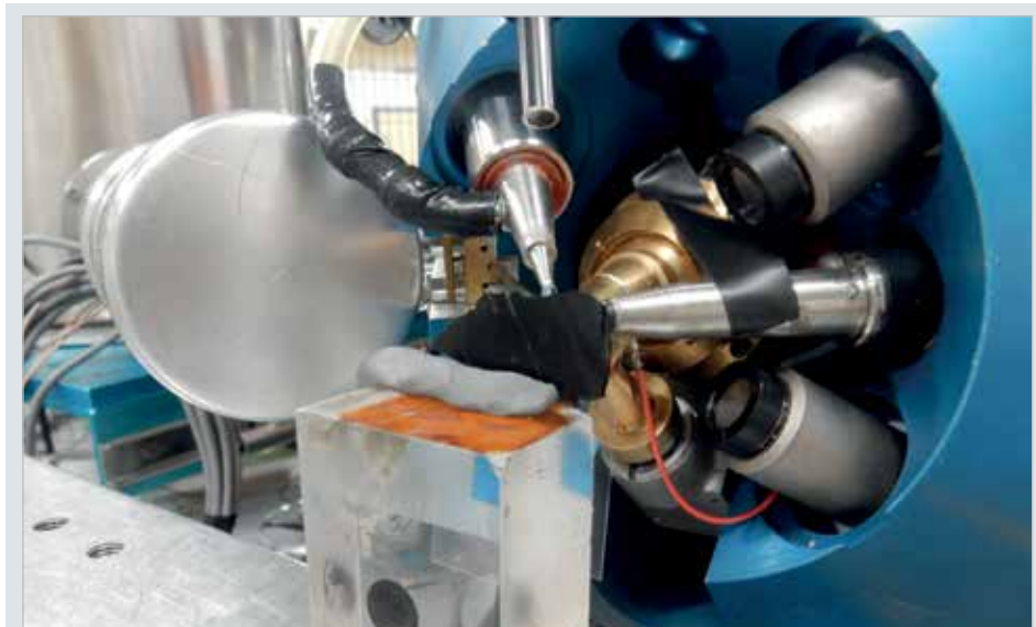
3: Photo shows Whitby Jet sample positioned in front of proton beam and detectors.
