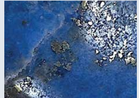
3: Pitted 'orange peel' surface of lapis lazuli, visible under oblique top illumination.
