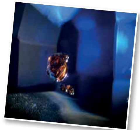
Mica crystal in an untreated burmese sapphire, taken with an iPhone 6s through an Eickhorst microscope with darkfield, magnification approximately 40x. Image by Sebastian Hänsel.
