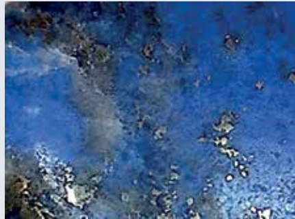
2: Polycrystalline nature of lapis lazuli, visible patches of calcite (left) and speckled pyrite minerals throughout.
