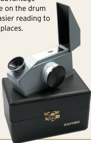
4: The Rayner Dialdex refractometer had a similar design to the original Rayner but with an external dial instead of the traditional internal scale.
