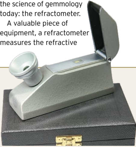
3: The Rayner had a sleek design for the era and featured a glass prism instead of a glass hemisphere.
