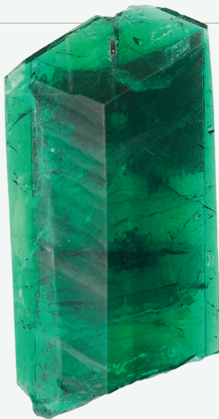
2: Synthetic emerald created using the hydrothermal method. Photo courtesy of Henry Mesa, Gem-A.
