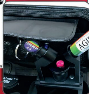
Smart UV Fluorescence adaptor & dark room
