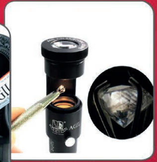
AGIL Polariscope Loupe detection of CVD Syn. Diamond
