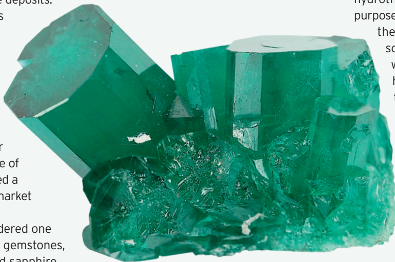
1. Synthetic emerald created using the flux-melt method. Photo courtesy of Henry Mesa, Gem-A.
