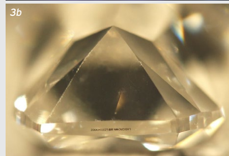
3a & 3b: 'Interrupted growth' banding resembles 'step facets' on this cushion modified brilliant cut CVD-grown diamond. It is interesting to note here is that if the fluoresce image on the left is observed on its own, it may appear growth bands are facet junctions instead.
