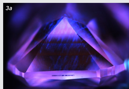
2a & 2b: CVD laboratory-grown diamonds with parallel fluorescent lines indicating the 'interrupted' growth process. They are running parallel to the table of the diamond. Blue luminescence is likely caused by structural defects.
