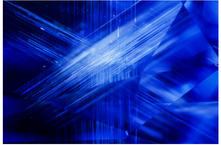
Elongate exsolution silk (i.e., tiny rutile needles) sometimes occurs in sapphires, as it does in this unheated Sri Lankan specimen. Field of view 2.00 mm.
