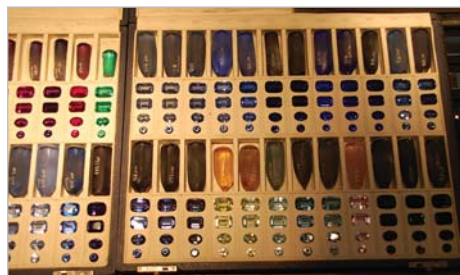
9: Some of the 37 different colours of Djeva's synthetic corundum production.
