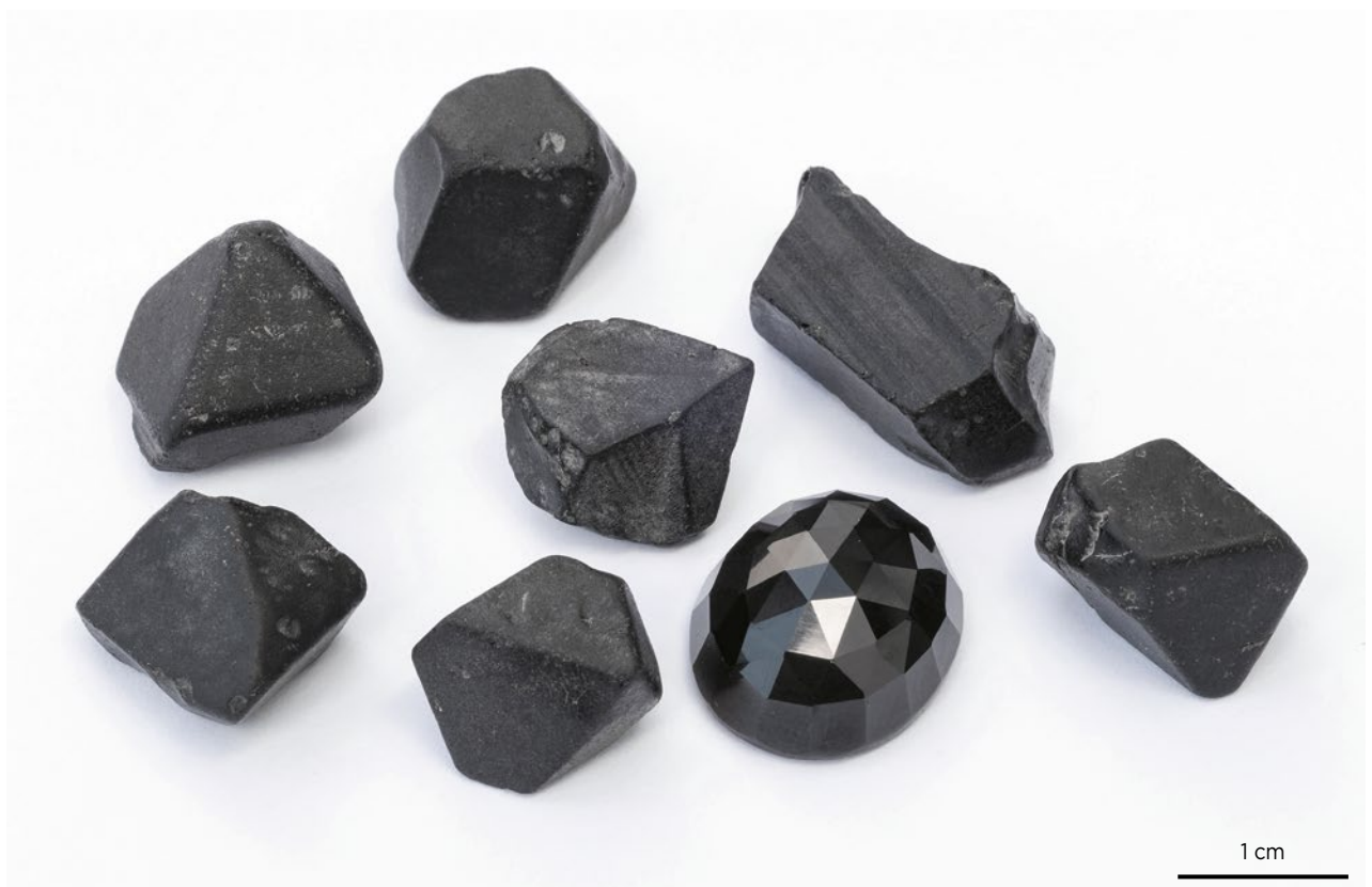
Figure 2: These seven crystals (4.8–6.7 g) and one faceted stone (32.7 ct) of black spinel are typical of material from Bo Phloi. The shapes of the crystals are dominated by octahedral faces, rarely in combination with rhombic dodecahedral faces (such as the top specimen). Some pieces (see, e.g., the one at the upper right) show surface striations. Photo by M. Wildner.
