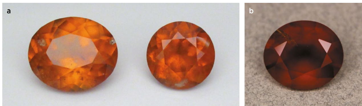
Figure 1: The Afghan hessonites examined for this report consist of (a) two medium orange gems weighing 6.41 and 3.85 ct, and (b) a deep reddish orange 10.49 ct oval. Photos by (a) B. Williams and (b) Dean Brennan, Stone Group Laboratories.
