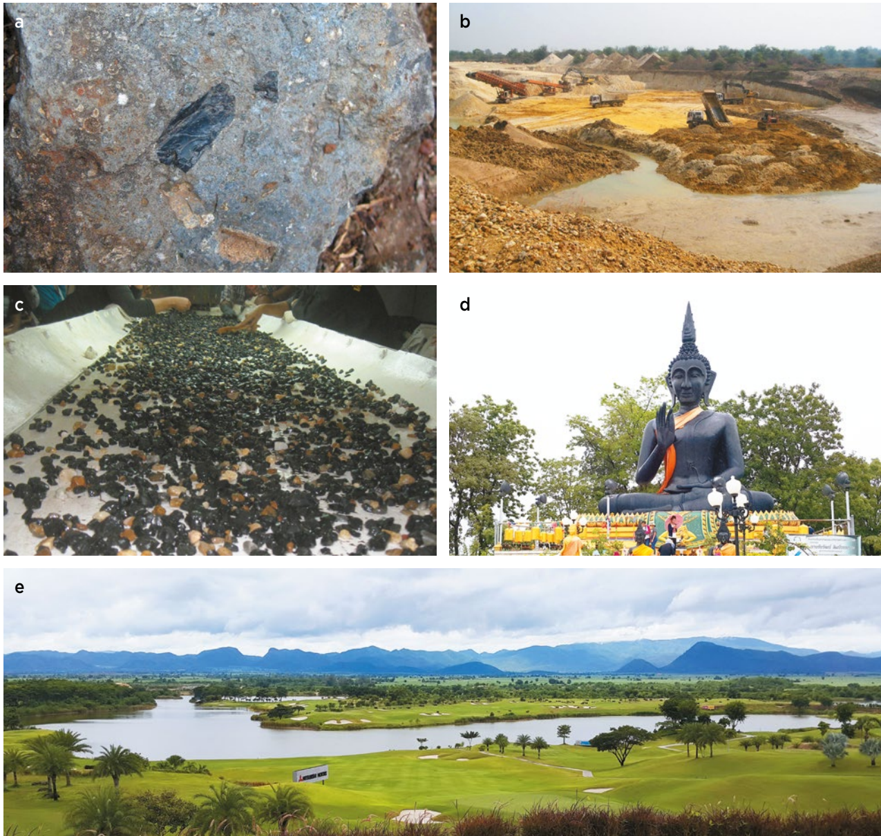
Figure 4: (a) Two spinel xenocrysts (16 mm and 5 mm long) are embedded in their basaltic host rock. (b) The sapphire and spinel mining site at Ban Bung Hua Waen, southwest of Bo Phloi, as seen in 2012. (c) Mine employees pick sapphires from a conveyor belt in March 2012. Most of the black material in this heavy mineral fraction consists of spinel, which was stockpiled. (d) This Buddha statue (Luang Por Nil) is located on a hill inside the town of Bo Phloi. It measures 9 m tall and is made from crushed black spinel mixed with cement. (e) This area along the Lam Ta Phoen River northwest of Bo Phloi hosted the former Ban Chong Dan mining area, which has been transformed into a golf course. Photos by B. Wanthanachaisaeng.
