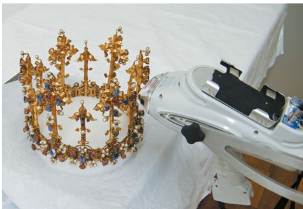
Figure 11: A portable EDXRF spectrometer was used to analyse constituents of the crown on site at the museum, initially with the piece in its circular state. Photo by K. Schmetzer, with permission to photograph and reproduce from Bayerische Schösserverwaltung, Munich.
