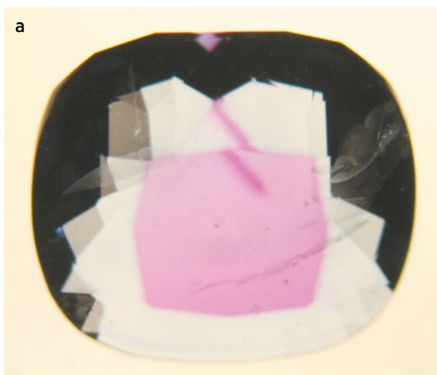
Figure 30: (a) Closer examination of the sapphire (immersed in water) shows pink colouration restricted to the table and along one portion of the pavilion. (b) At higher magnification (here, 22 \times ), the deep pink area on the pavilion can be seen to penetrate slightly below the surface of the stone, as expected for Cr diffusion treatment. Photomicrographs by B. Williams.
