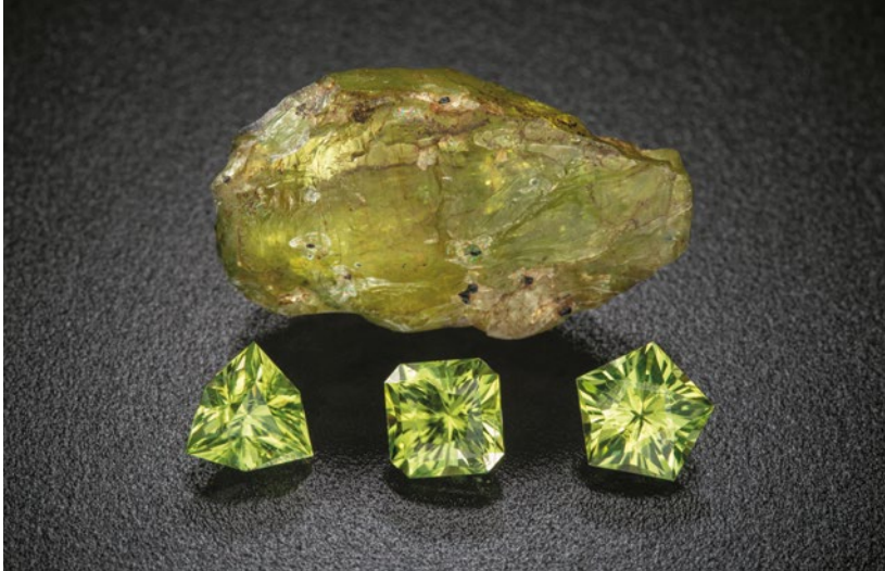
Figure 11: South-central British Columbia, Canada, has produced small amounts of gem-quality peridot with good colour but typically in small sizes. Shown here is a rough piece (2.5 cm wide) from Lightning Peak and three faceted stones (1.1–1.25 ct) from the northernmost peridot-producing locality in Figure 6. Further gem exploration of basaltic terranes in this region using the remote-sensing techniques described in this article could result in additional production of gem-quality peridot. Photo by Michael Bainbridge.
