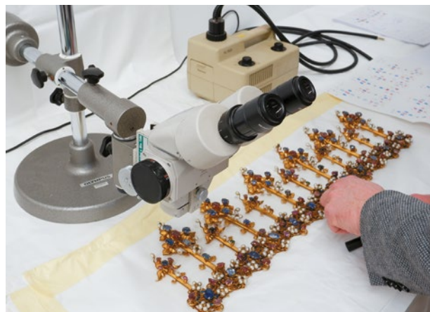
Figure 13: The flattened geometry of the opened crown facilitated microscopic examination of the 12 base segments and fleurons and allowed the individual gem materials to be more easily targeted by the EDXRF spectrometer (not shown here). Photo by K. Schmetzer, with permission to photograph and reproduce from Bayerische Schösserverwaltung, Munich.
