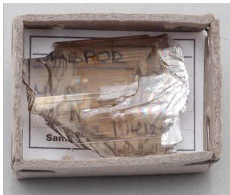
1: A rough diaspore crystal (4.5 cm length) from Turkey, with a light colour change due to 0.1 wt.% Cr 2 O 3 .
