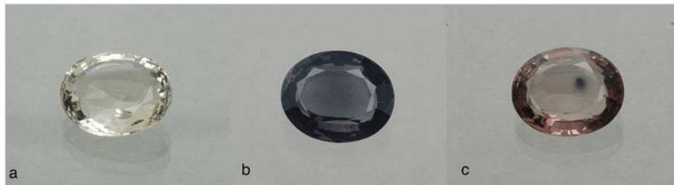
Photochromatic glass imitating a gemstone. The stone is light yellowish in normal light (left), dark bluish grey after exposure to a strong light source (middle) and slowly fades back after a few hours in the dark safe (right) showing brownish hues before returning into its original light yellow colour. This stone which was sold as an 'extraterrestrial stone of heaven' is actually a very common artificial glass product, normally used for sunglasses or sun-protecting windows of buildings. © M.S. Krzemnicki, Swiss Gemmological Institute.
