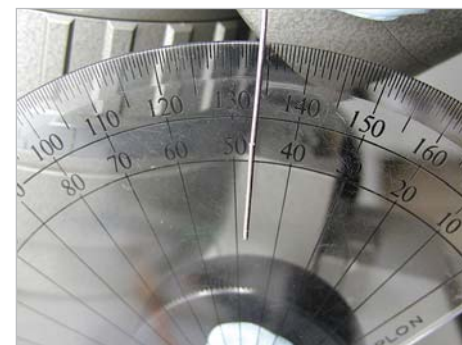
4: Paperclip with 'double' pointer (left), showing line of vision is set for all readings (right).
