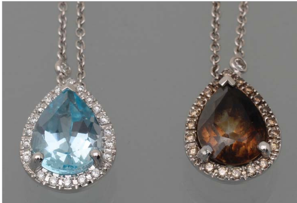
Irradiated blue topaz (left) as it was sent to an SSEF client and how it was returned (right) after a few weeks. The brownish colour of the topaz is due to a coating with rust, perhaps because it fell into the client's barbecue. © M.S. Krzemnicki, Swiss Gemmological Institute SSEF.
