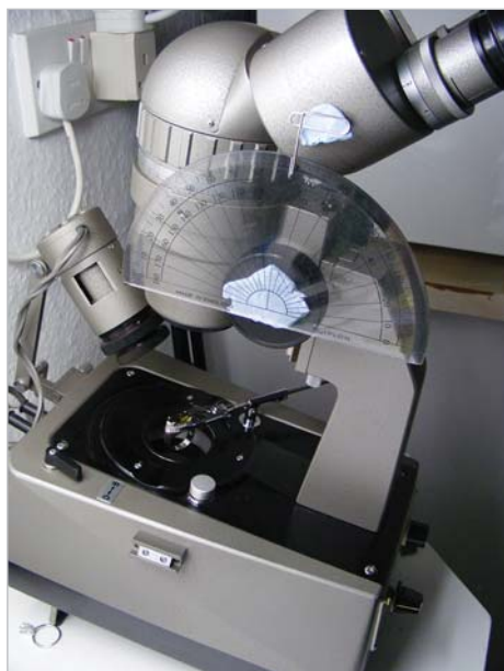
3: Microscope focus knob with protractor tacked on.
