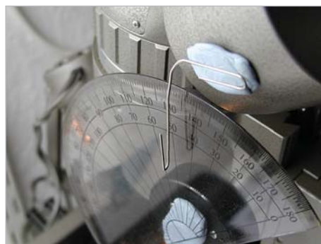
4: Paperclip with 'double' pointer (left), showing line of vision is set for all readings (right).
