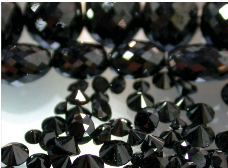
1: Most of what you see at JCK are the heat-treated black diamonds shown here — round brilliant cuts and faceted beads. The poor quality starting material is always evident under magnification and even here in the image — you can see pits, cavities and fracture lines on many of these random samples. Obviously, these gems are admired for their colour and their lustre (adamantine). Courtesy of Danis GMBH, Tiefenbronn, Germany.
