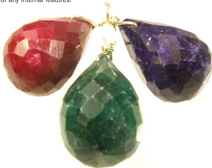
5: These dyed corunda were originally greyish in colour. CCF reactions were the opposite of what would be expected based on appearance.
