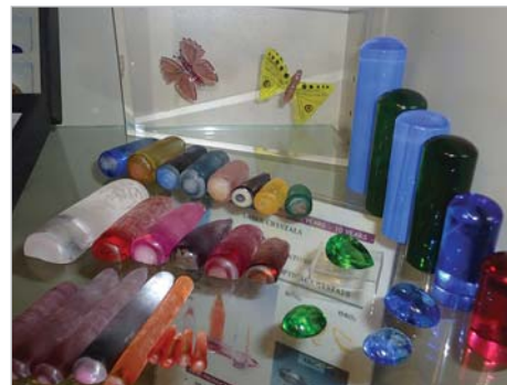
Left and above: synthetic boules created at the Forschungsinstitut . The rods are cut from the boules and used in various laser applications. Images Olga Gonzalez.
