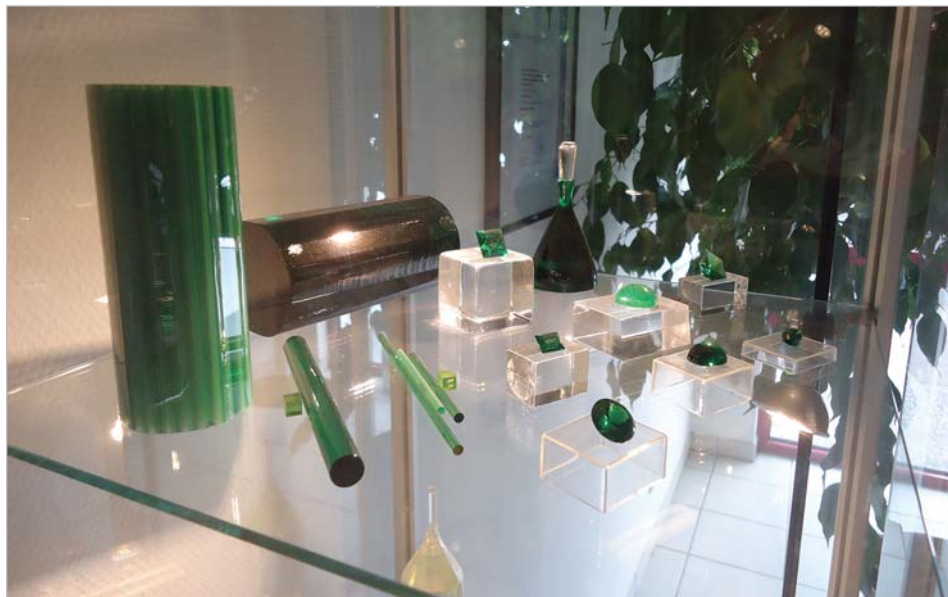
Left and above: synthetic boules created at the Forschungsinstitut . The rods are cut from the boules and used in various laser applications. Images Olga Gonzalez.
