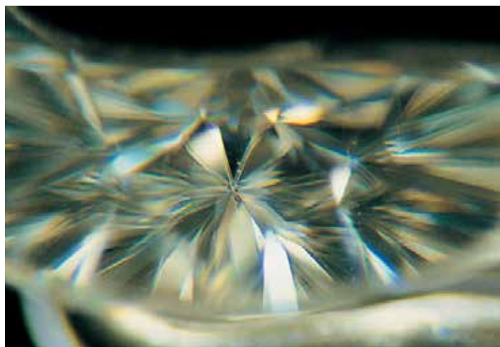
Doubling of back facets in synthetic moissanite.
