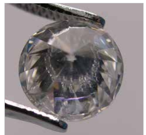
21: Diamond (1.08 ct) seen from slightly different angles, displaying purple flash of a filled cleavage fracture. Magnification approx. 7x.
