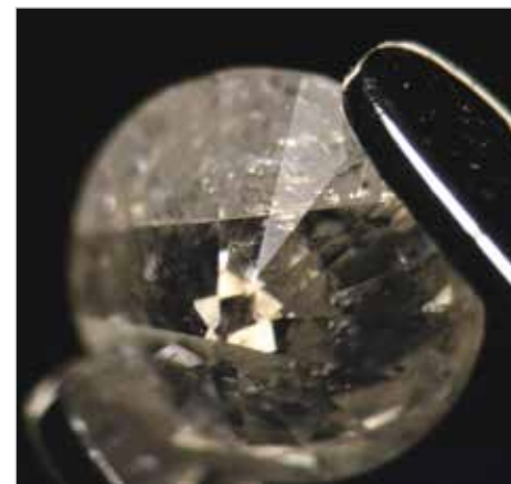
9: Diamond, 0.17 ct, viewed from the pavilion side, showing a cleavage plane extending across the whole of the stone.
