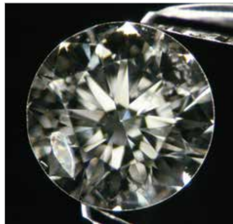
4: A cleavage, although from the pavilion surface, can be seen through the crown, giving a piqué 1 or Included 1 (I1) clarity grade.
