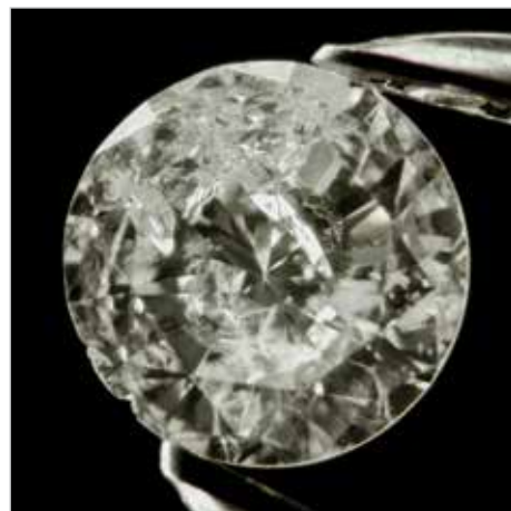
3: Cleavage fractures of all sizes are present in this diamond and they are also responsible for the nicks in the girdle (bottom left).
