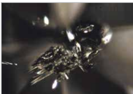
2: This central black 'spot' was seen to be a cluster of graphite-lined cleavage discs. Magnification approx. 60x.
