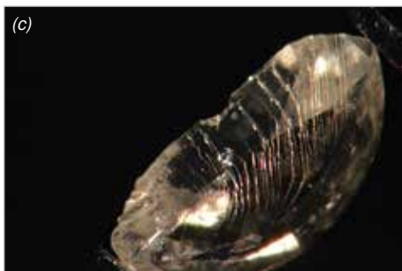
10: A brilliant-cut diamond, 0.56 ct, after being cleaved during setting. (a) Two views of the diamond, (b) the larger portion, (c) the smaller portion (the bottom left of this piece fits against the top right piece of (b)), and (d) the main cleavage face, as seen in (b), is shown in the dark area across the right of this picture. Look at the stepped effect shown in two areas on the table surface. Magnification approx. 80x.
