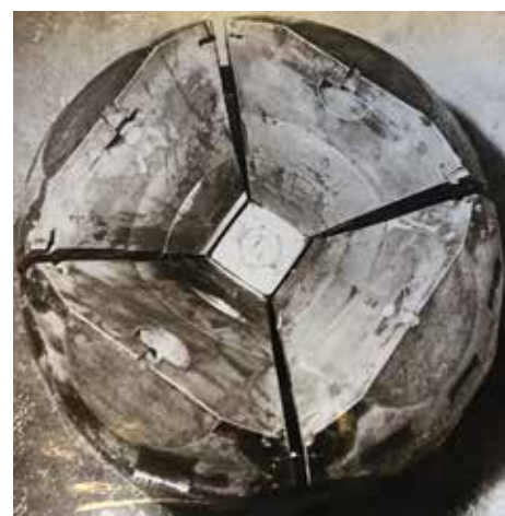
Right: The sphere when sealed and put under hydrostatic pressure. Photos Swedish National Museum of Science and Technology.
