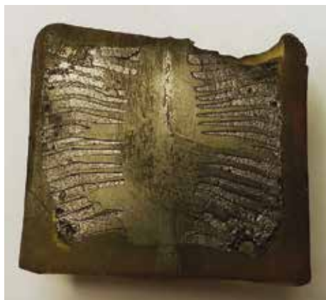
The reaction chamber cut in half and moulded in plastic for preservation at the Swedish National Museum of Science and Technology. Diamonds grow between the dark layers of cobalt. Photo Jan Asplund.
