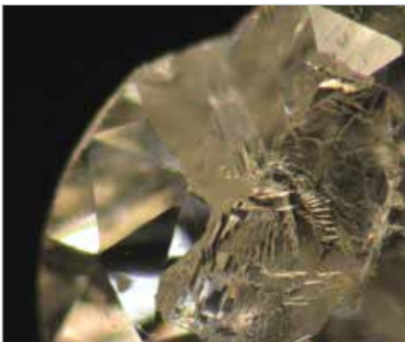
14: Extensive cleavage terraces plus a missing section are the result of a force applied to this 0.11 ct diamond.
