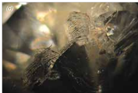
10: A brilliant-cut diamond, 0.56 ct, after being cleaved during setting. (a) Two views of the diamond, (b) the larger portion, (c) the smaller portion (the bottom left of this piece fits against the top right piece of (b)), and (d) the main cleavage face, as seen in (b), is shown in the dark area across the right of this picture. Look at the stepped effect shown in two areas on the table surface. Magnification approx. 80x.
