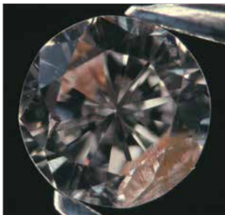
7: Large cleavage fracture situated just below the girdle which contains reddish iron staining (lower right). Notice the reflection of this on the opposite side.
