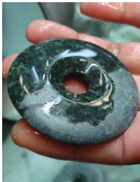
7: Final sanding stage on a disc of 'Mayan Foliage' jade — a very popular green and white mottled variety, at the Jade Maya™ shop in Antigua.
