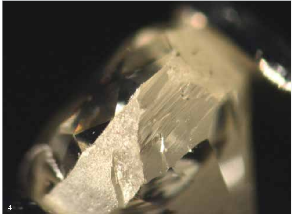
4: Large 'natural' of parallel striations, magnification approx. 80×.
