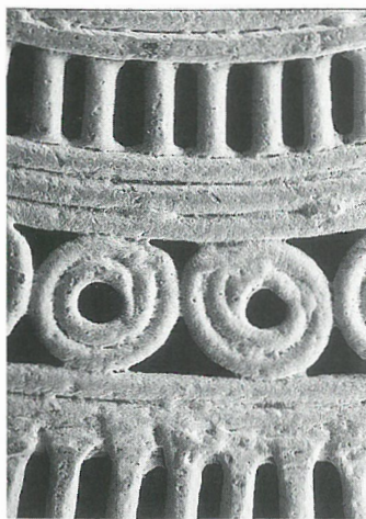
Magnified scanning electron microscope image of the 'false filigree' construction of the earrings which preserves the plastic form of the original wax model and the typical dendritic texture of casting. Photo courtesy of British Museum Department of Scientific Research.
