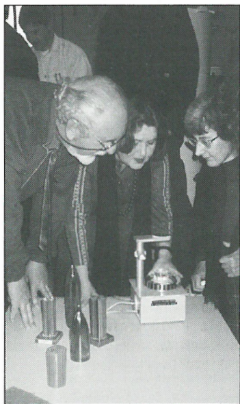
At the Research Institute: Robert Brunt, Merle Thackrah and Christine Woodward examine slices of the synthetic boules under the polariscope.
