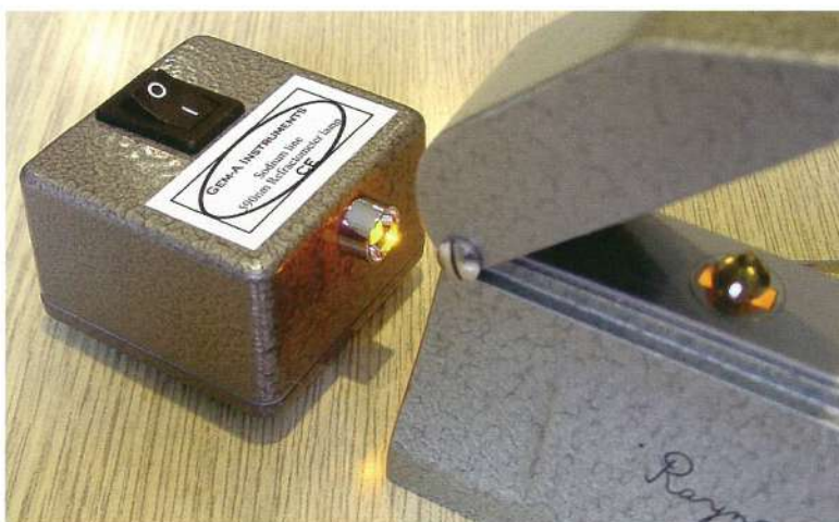
The portable lamp in use with a Rayner refractometer.
