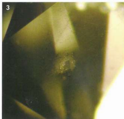
Magnified view of the sapphire showing a 'space nebula' cloud of very small gas bubbles, with a few slightly larger ones.
