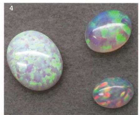
The 12 x 10 mm test stone on the left; Gilson synthetic water opal upper right; modern synthetic opal (unknown manufacturer) lower right.
