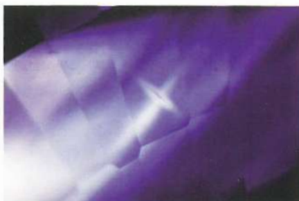
An excellent example of chromophore consumption is shown by the colourless zone surrounding the minute inclusions in this unheated blue sapphire. The exact opposite of internal diffusion which proves treatment, chromophore consumption, as shown by colour depleted zones around inclusions, provides excellent microscopic proof of natural colour. Photomicrograph by John I. Koivula, courtesy of microWorld of Gems.
