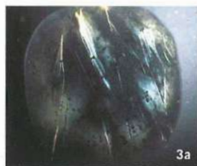
The synthetic spinel at different positions under the polariscope.
