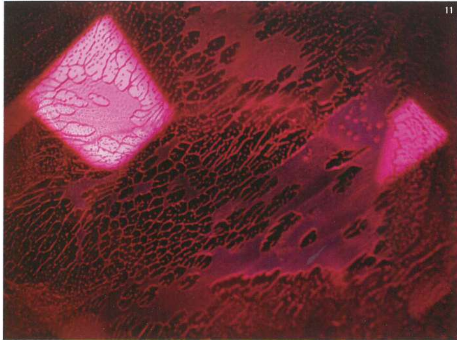
Microscopic indications for glassy residues may exist in round droplets, channels with drop-like extensions or turbid films.
