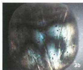
The synthetic spinel at different positions under the polariscope.
