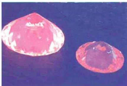
Fluorescence under UV light: the natural type II left and a CVD synthetic diamond right.
