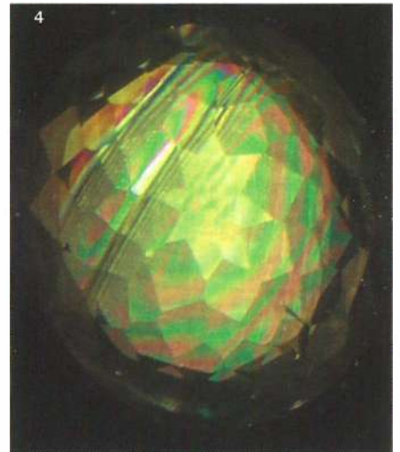
The stone under crossed polars, showing interference colours and the two twin planes.
