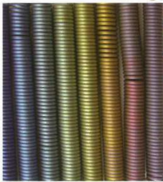
Anodised titanium wire spirals (inset) showing the mid-range of interference colours, subsequently cut to form the links of the tubular chain mail bracelet. Lynne Bartlett, 2005.
