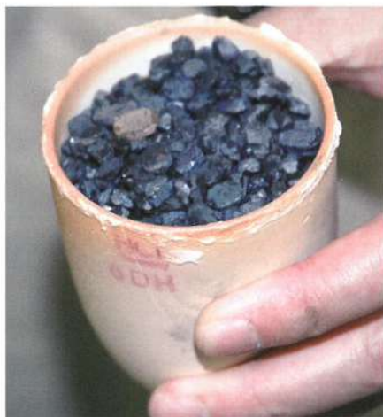
Crucible containing heat-treated sapphires using the traditional methods.
