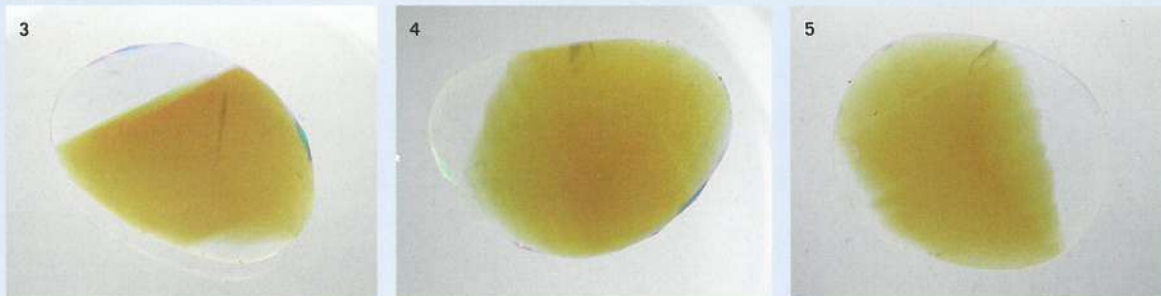
The sapphire immersed in methylene iodide showing three different positions.
