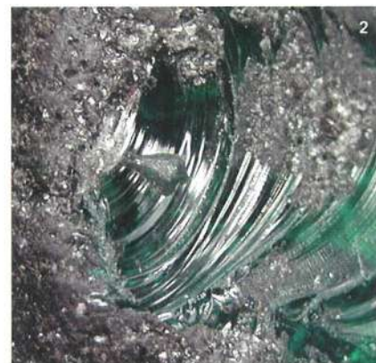
Glass 'emerald' showing epoxy resin teardrop.
