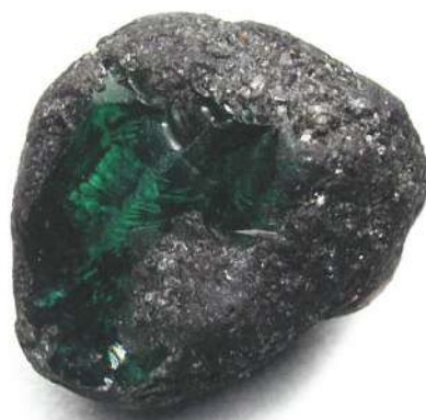
Glass 'ruby' and 'emerald' crystals. The 'ruby' sample appears to have brick dust particles in the coating.
