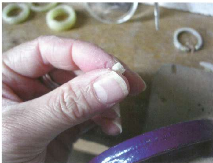
Carving the bioglass into a ring shape.
