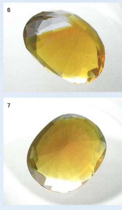
The sapphire immersed in toluene (RI 1.49).
