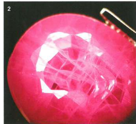
Quench-crackled flame-fusion synthetic rubies with healed fractures (1, 2 and 3). The original curved growth lines have been retained (1) and several stones show coarsely filled fractures (3).
