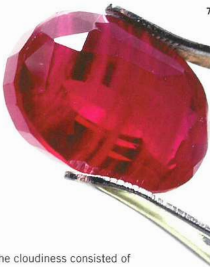
6 One of the stones shown in 5 seen from different angles. In 6 the bubbles appear to be just clouds giving the stone a translucent look, but viewing the same stone from a different angle shows the broad, curved nature of the bubble clouds (7).
