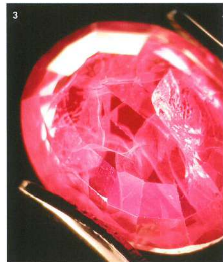
Quench-crackled flame-fusion synthetic rubies with healed fractures (1, 2 and 3). The original curved growth lines have been retained (1) and several stones show coarsely filled fractures (3).
