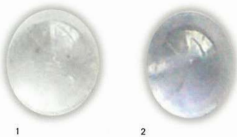
Sri Lanka corundum (1) heat-treated with beryllium and other additives at 1750°C for about six hours and (2) heat-treated for 50.
