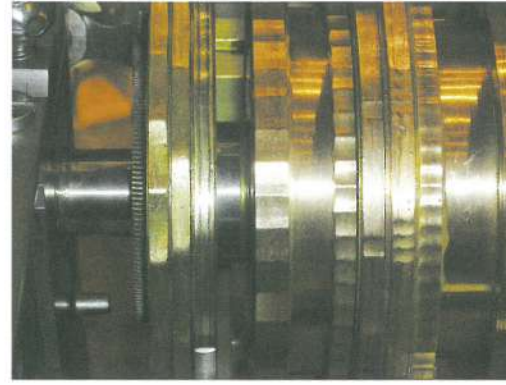
5. The heart of the engine turning machine – geared wheels that can be rotated in a vast number of configurations to produce the intricate geometric designs.
