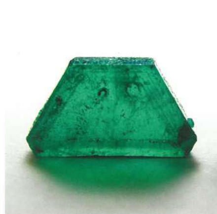
1. Tabular crystal of Lennix synthetic emerald, width 17.3 mm, weight 6 ct. © Gem-A.
