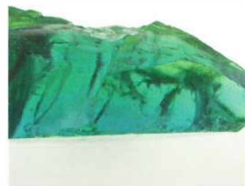
2c and d: A rough glass specimen with a misleading appearance of displaying pleochroism.
