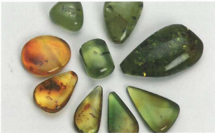
1 Treated Colombian copal. The green samples have received more treatments in an autoclave than the golden material. Photo © Maggie Campbell Pedersen.
