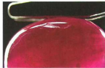
2 The filled section of the ruby. Magnification 20x.
