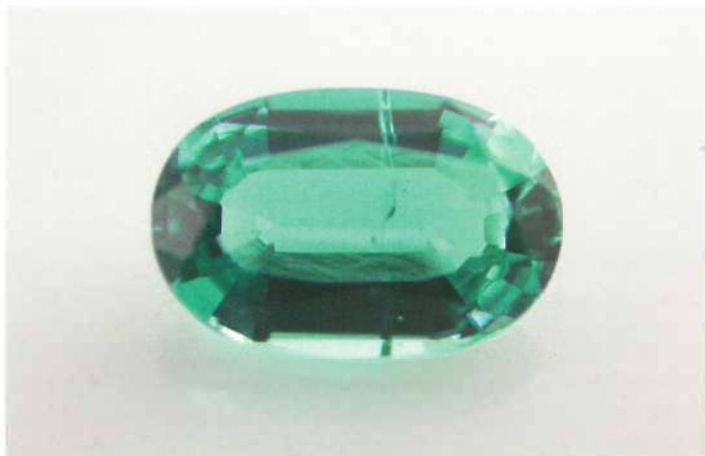
2c and d: A rough glass specimen with a misleading appearance of displaying pleochroism.
