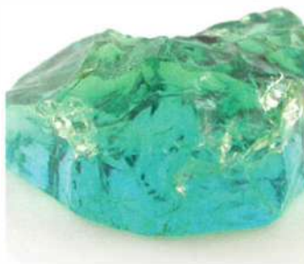
2c and d: A rough glass specimen with a misleading appearance of displaying pleochroism.
