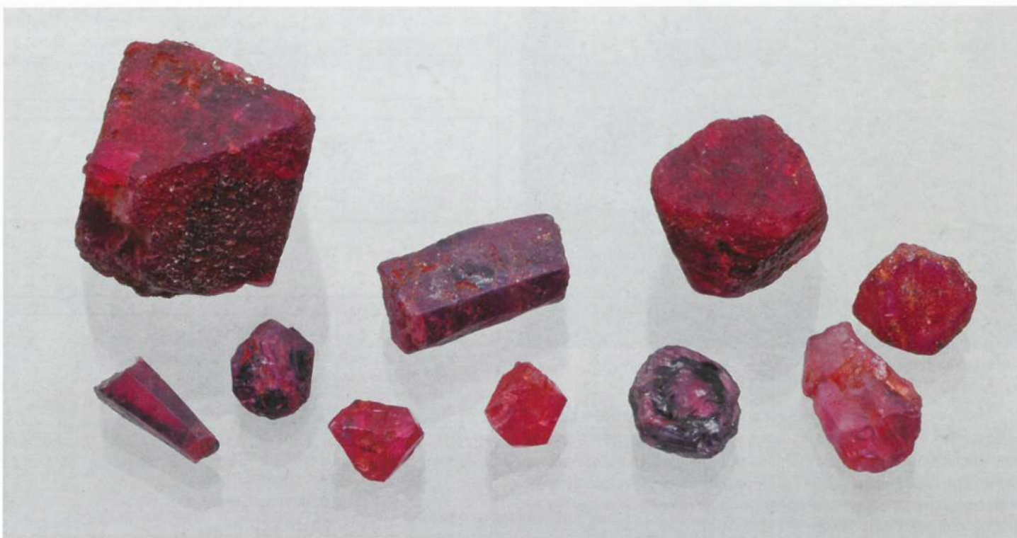
Fig. 6: Ruby crystals of rhombohedral to prismatic habit from Winza, Morogoro Area, Central Tanzania. The largest stone is 25 mm across and 88 ct. Photo © H.A. Hänni, SSEF Swiss Gemmological Institute
