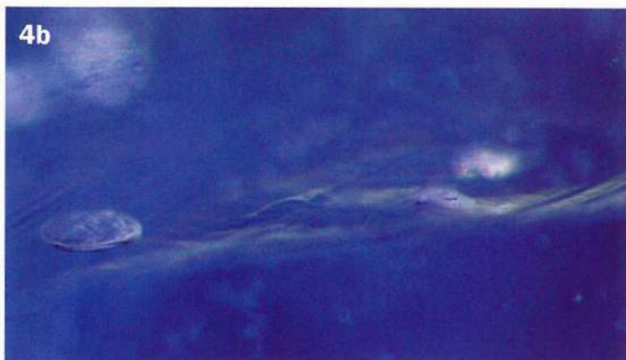
4 (a and b). The internal features of the lead-glass-treated blue sapphires: a few flattened gas bubbles and/or glass relicts and faint to weak green to yellow interference colour in the filled cracks.
