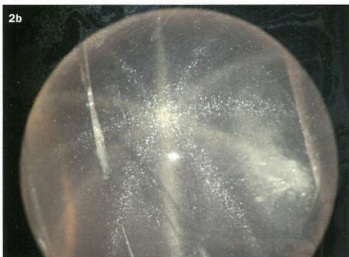
The 49 mm sphere (2) in water, epiasterism, and 3 in air, diasterism, a and b showing opposite poles.
