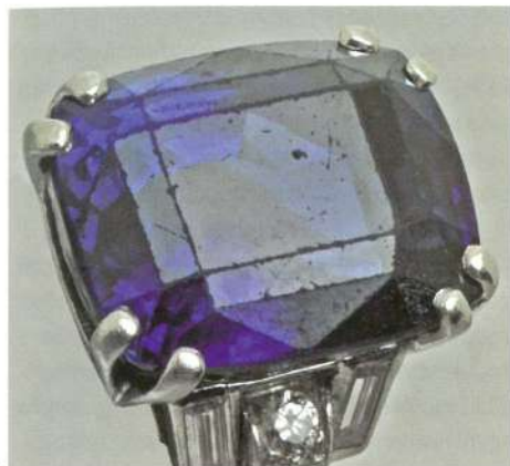
8. Wear marks on a sapphire mounted in a ring, with abrasions on facets, corners and edges.
