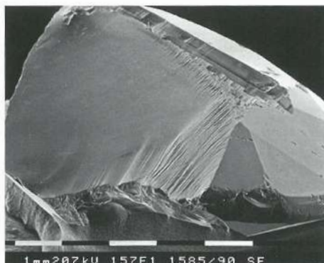
14. SEM picture showing the break structure of a sapphire damaged during enlargement of a ring. The force to break the stone comes from the culet and after a conchoidal break it ends in a stepped structure near the table of the stone. Length of white bar 1 mm.
