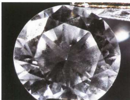
6. A soldering repair to a ring containing this 0.30ct brilliant cut diamond left the stone with a totally burned surface.
