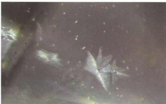
Dendritic crystallites in a glass-filled fracture
