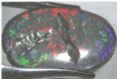
19. To re-size or deform a ring may put considerable stress on a stone in a closed setting. This flat black opal cabochon broke when the goldsmith re-adjusted the ring.
