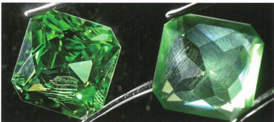
16. The warm acid bath used after repair soldering has attacked the surface of this peridot; distinct corrosion is visible after only 20 minutes, making the surface matt. (a) Original peridot (b) after 20 minutes in pickling solution.
