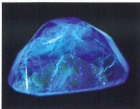
15. Fissure-filled emerald seen in LWUV illumination. The extended network of bright lines shows a significant degree of treatment. The whitish fluorescence of the filler is typical for epoxy resin. Length of the stone approx. 12 mm.
