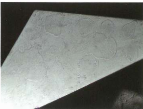
5. Burned surface spots (burn marks) on a star facet of a brilliant cut diamond. Magn. 30x.
