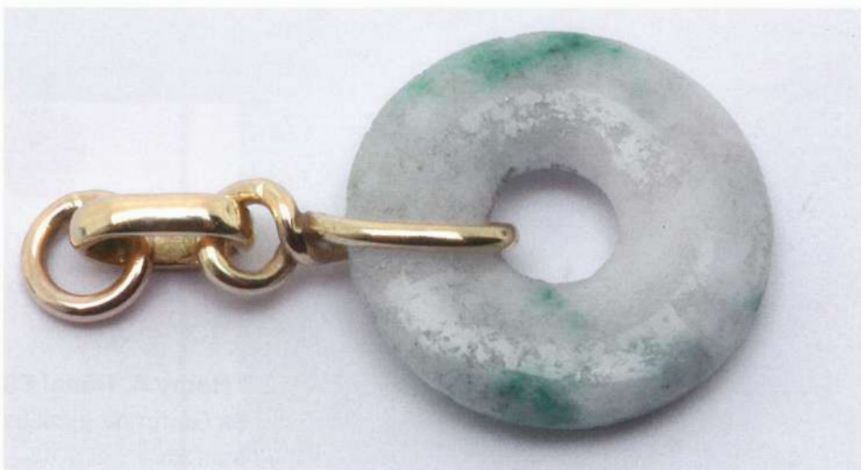
18. A B-jade pendant with a rough surface after ultrasonic cleaning. The porous structure is due to disintegration of the impregnated material.
