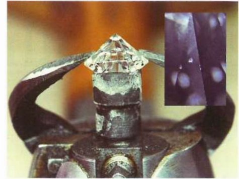
4. Forced closing of the claws of the dop for pavilion facet cutting may cause pressure marks. Such fissures may be visible at 10x and affect the clarity grade.
